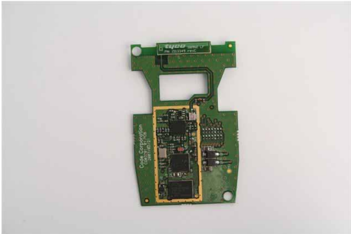
Photograph 4 - Component Side of PCB with RF Shield Removed
