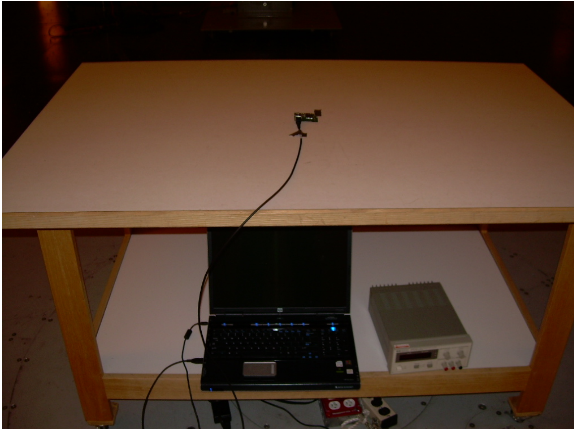
Photograph 2 - Back View of the Radiated Spurious Emission Setup
