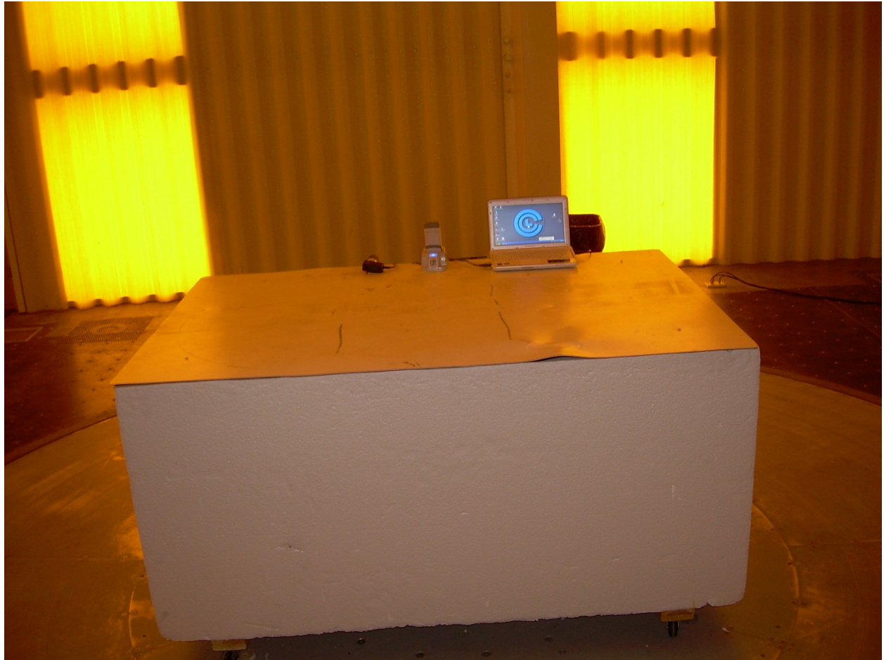
Front View Radiated Disturbance Worst Case Configuration
