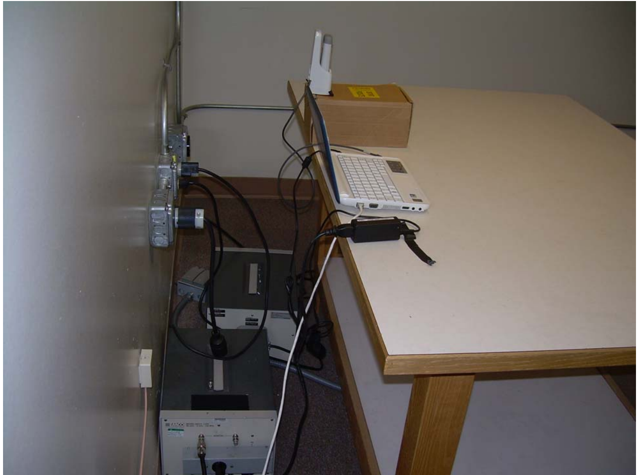
Back View Conducted Disturbance Worst Case Configuration
