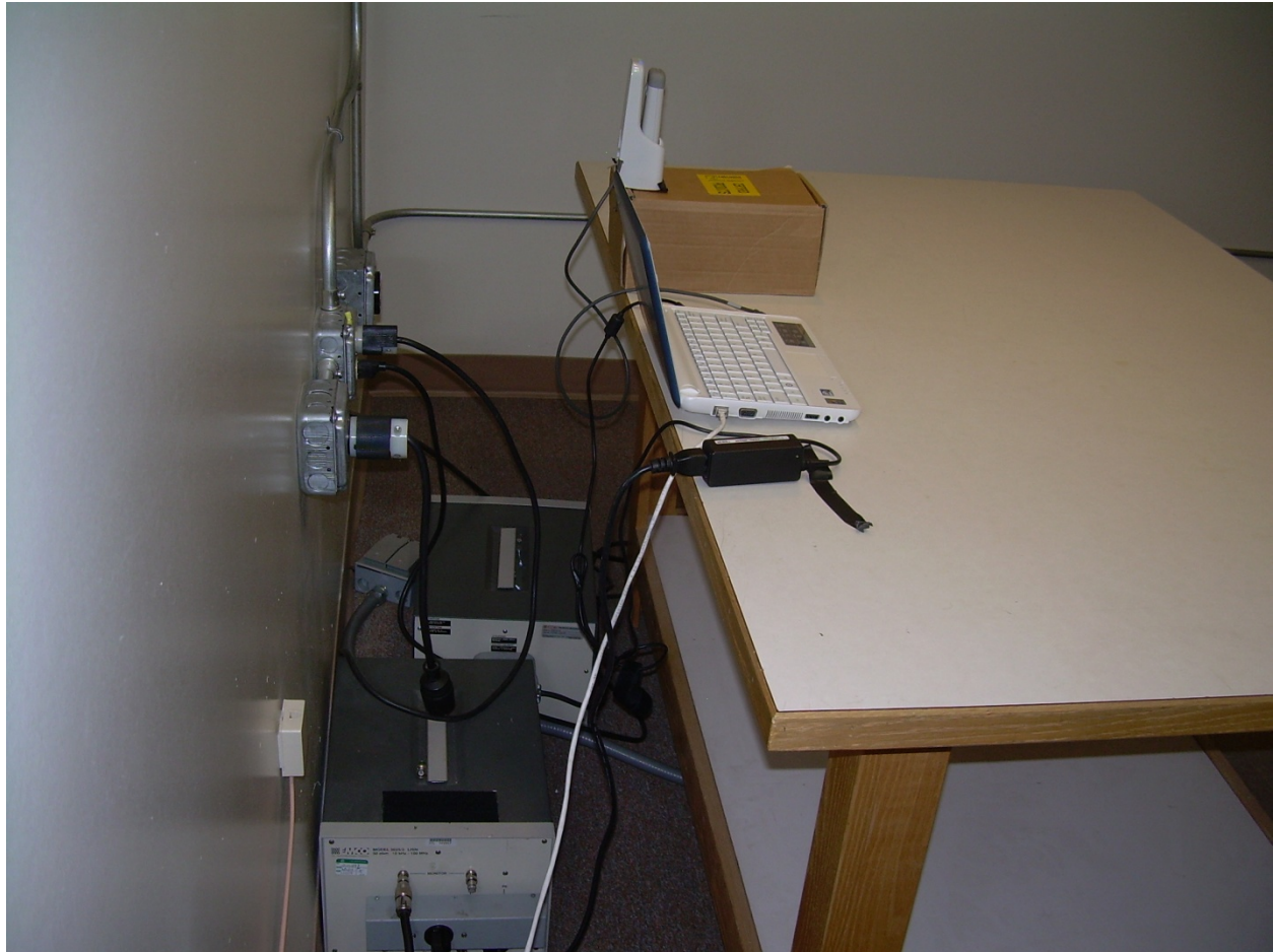
Photograph 4 – Back View Conducted Disturbance Worst Case Configuration
