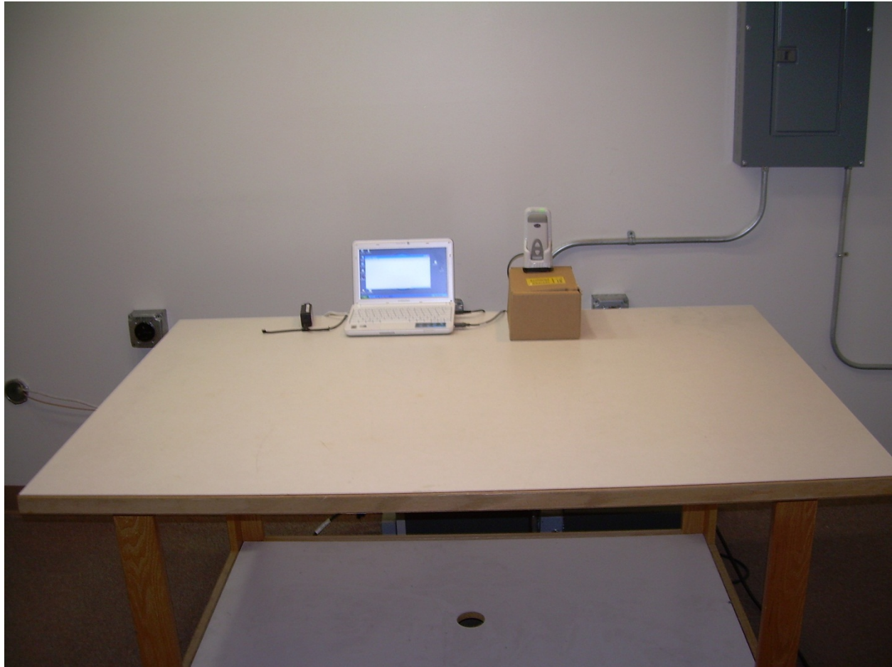
Photograph 3 – Front View Conducted Disturbance Worst Case Configuration
