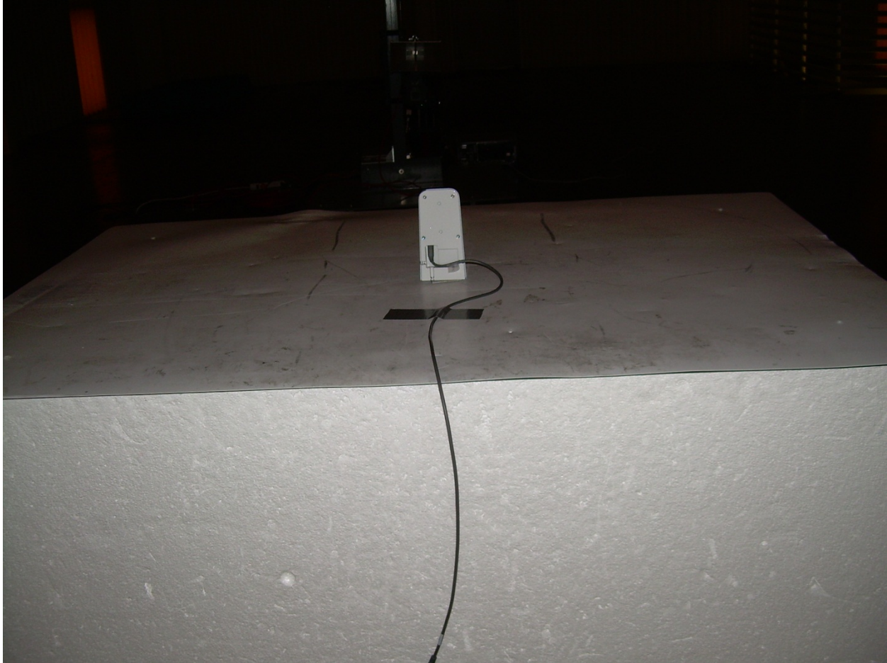
Photograph 2 – Back View Radiated Disturbance Worst Case Configuration
