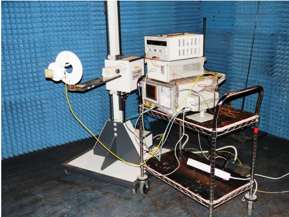
Photograph for Radiated Emission Test Setup/ 1
