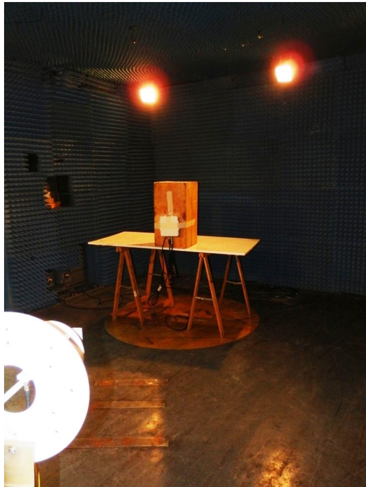
Photograph for Radiated Emission Test Setup/ 2
