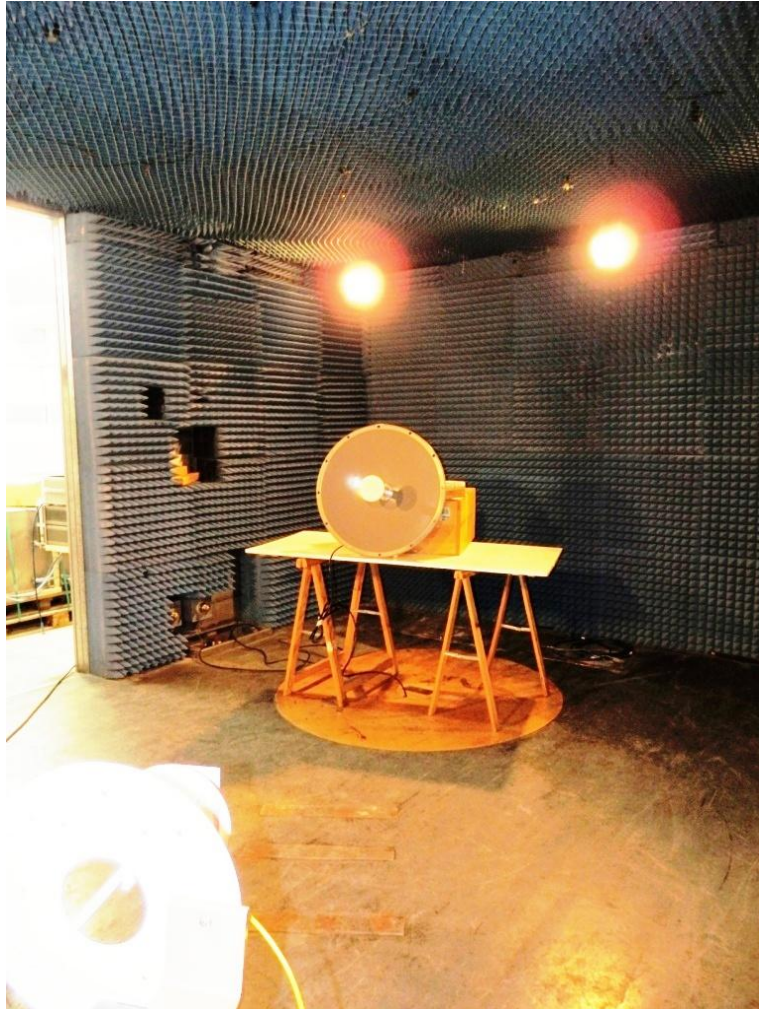
Photograph for Radiated Emission Test Setup/ 3
