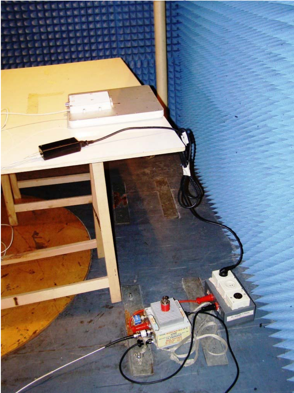
Photograph of Conducted Emission Test Setup/ 1
