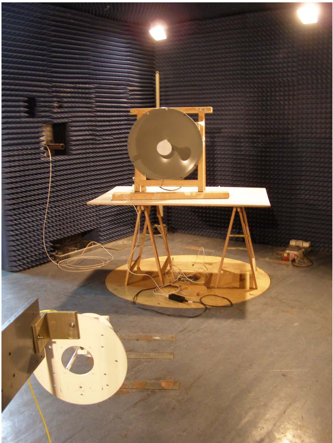
Radiated Emission Test Setup – Dish Antenna
