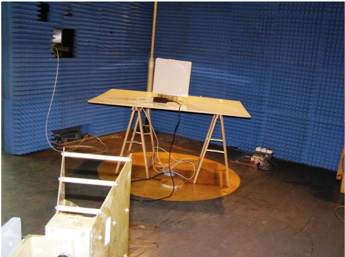
Radiated Emission Test Setup
