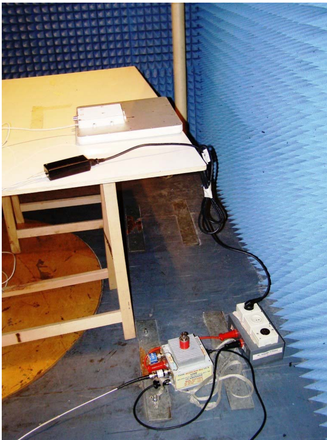
Conducted Emission Test Setup
