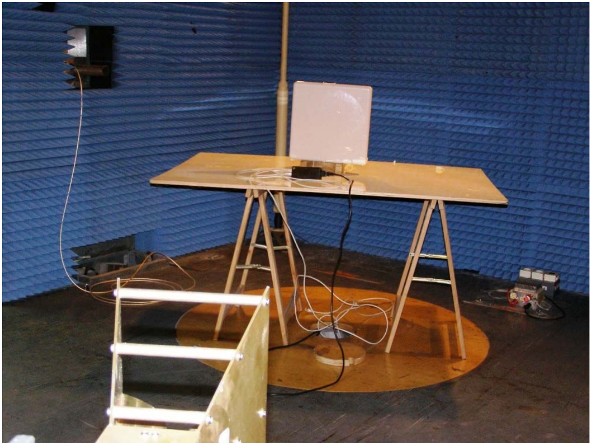
Radiated Emission Test Setup
