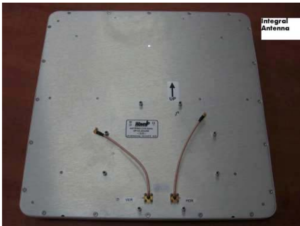
23dBi Integral antenna back side
