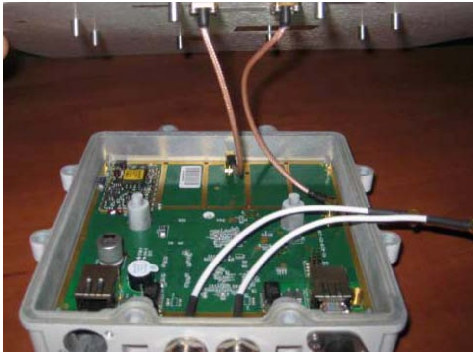
Internal picture with integral antenna connection
