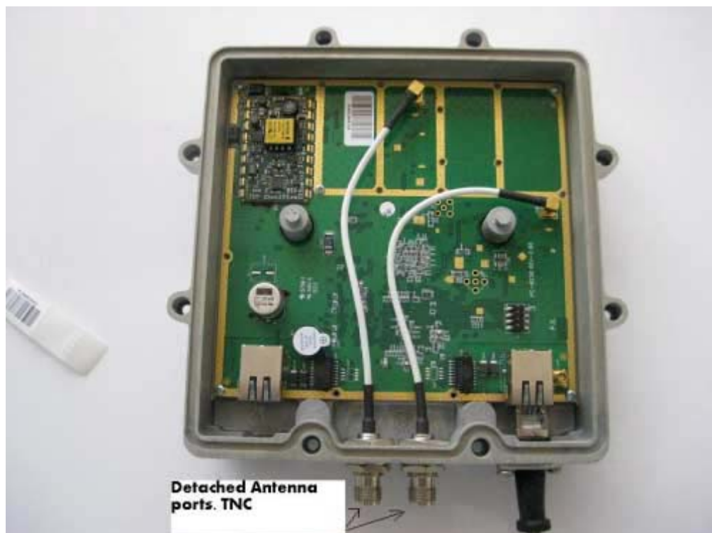
Internal picture with detached antenna ports (TNC connectors)
