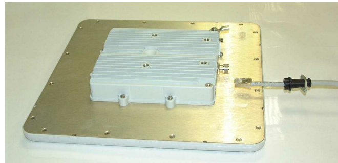
Figure 2-7: Cable insertion to Outdoor Unit.
