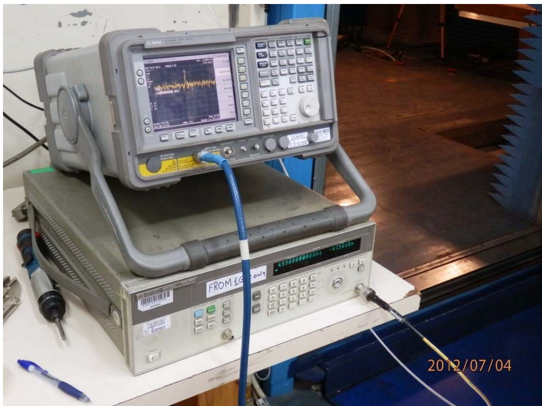
Photograph for Substitution of ERP Test Setup
