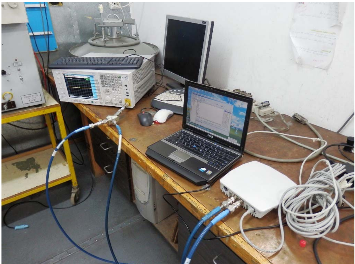
Conducted Measurement Test Setup
