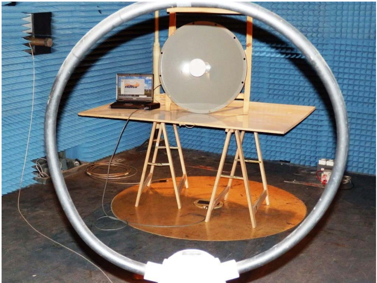
Radiated Emission Test Setup
