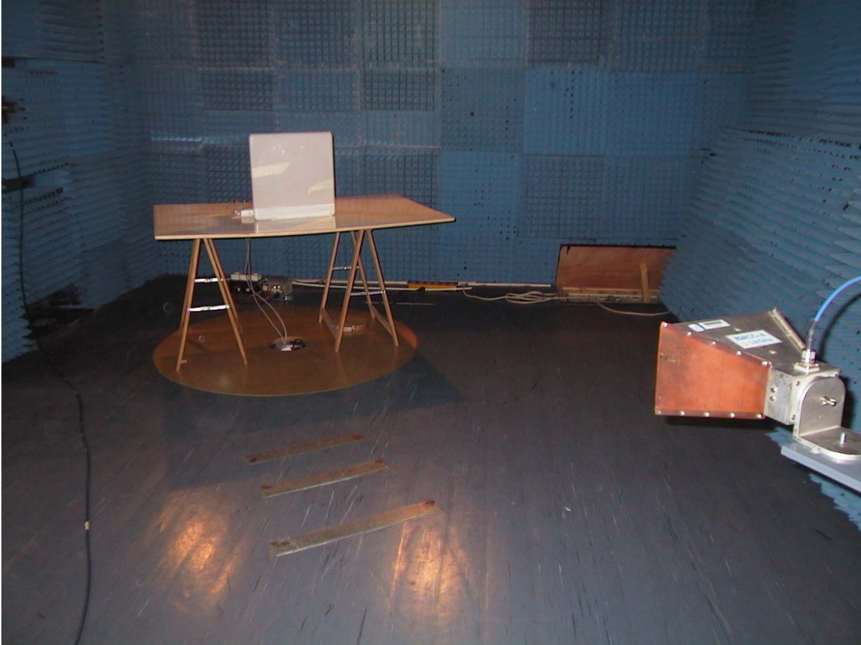
Radiated emission 1GHz – 18GHz Setup
