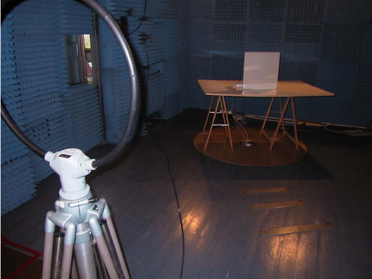
Radiated emission up to 30MHz Setup
