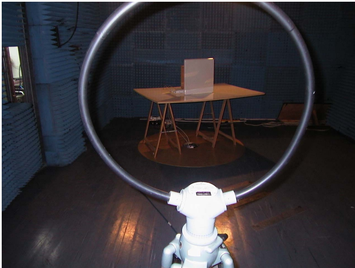
Radiated emission up to 30MHz Setup
