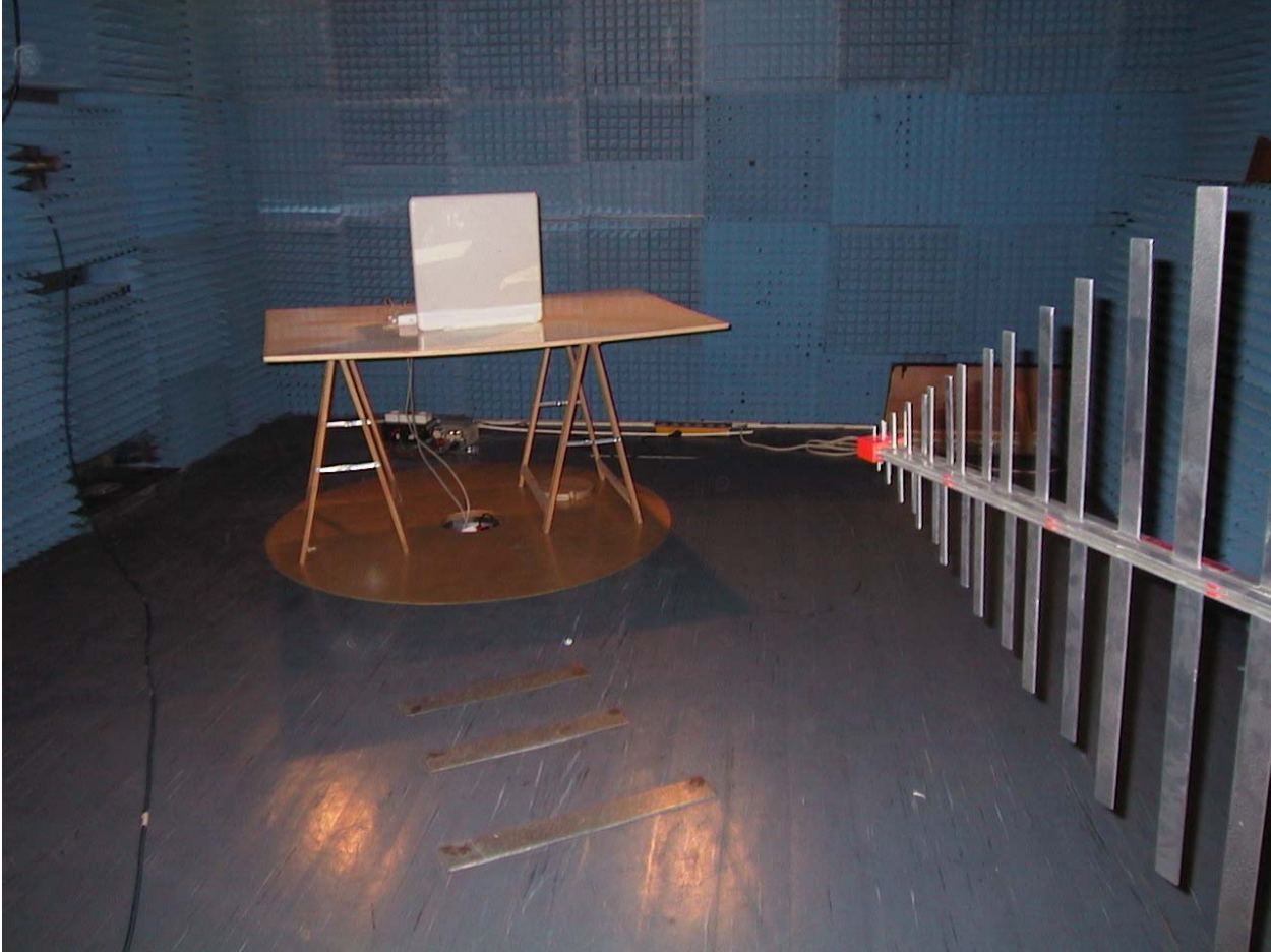
Radiated emission 30MHz – 1GHz Setup
