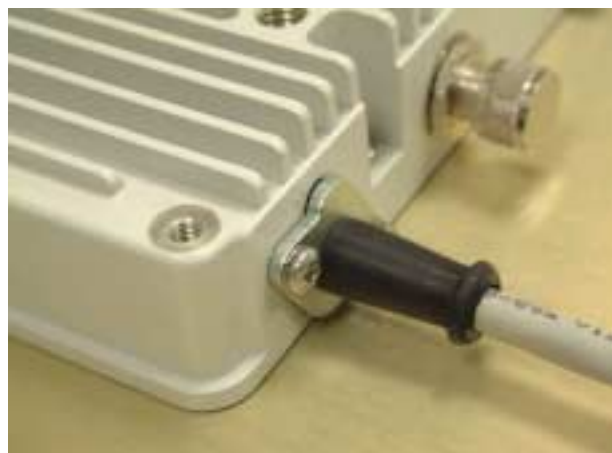
Figure 2-7: Cable connection to Outdoor Unit
