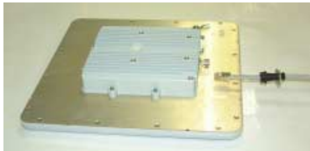
Figure 2-6: Cable insertion to Outdoor Unit.
