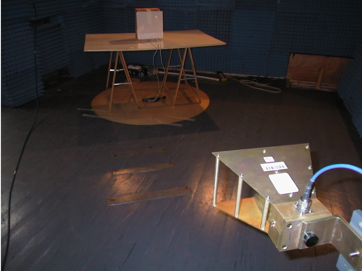
Radiated emission 1GHz – 18GHz Setup
