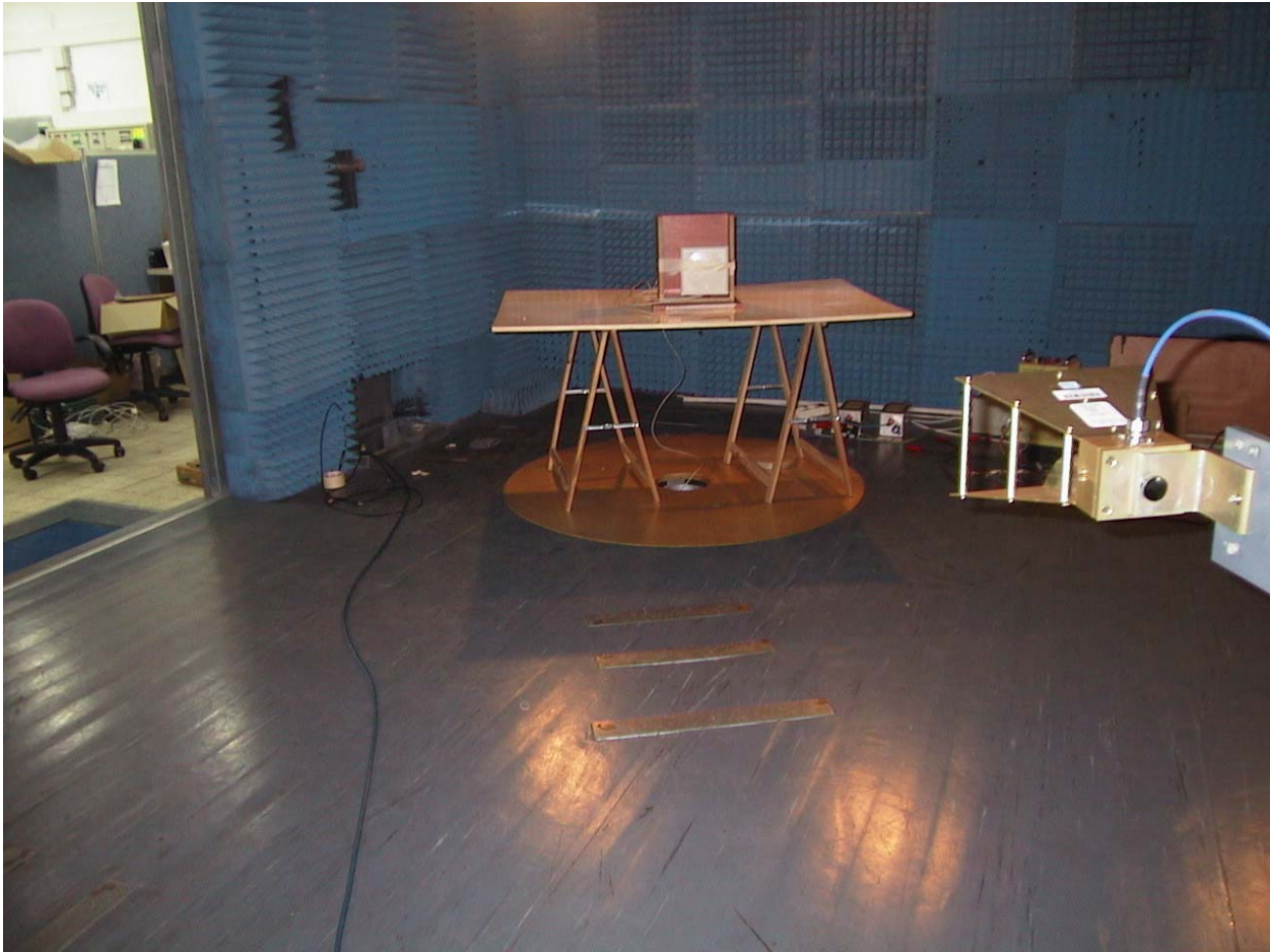
Radiated emission 1GHz – 18GHz Setup
