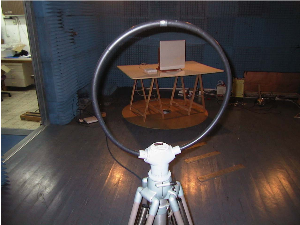
Radiated emission up to 30MHz Setup
