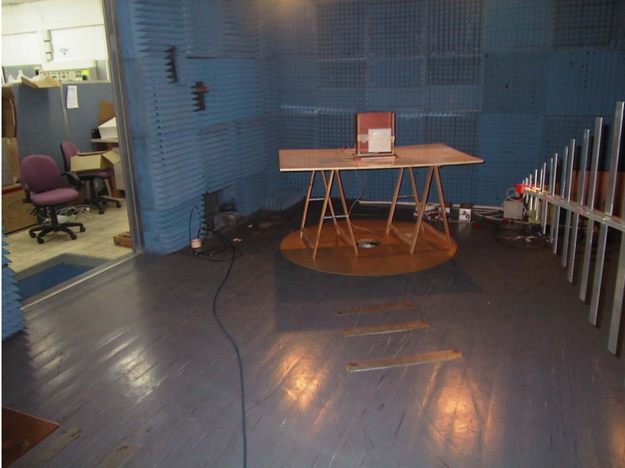
Radiated emission 30MHz – 1GHz Setup
