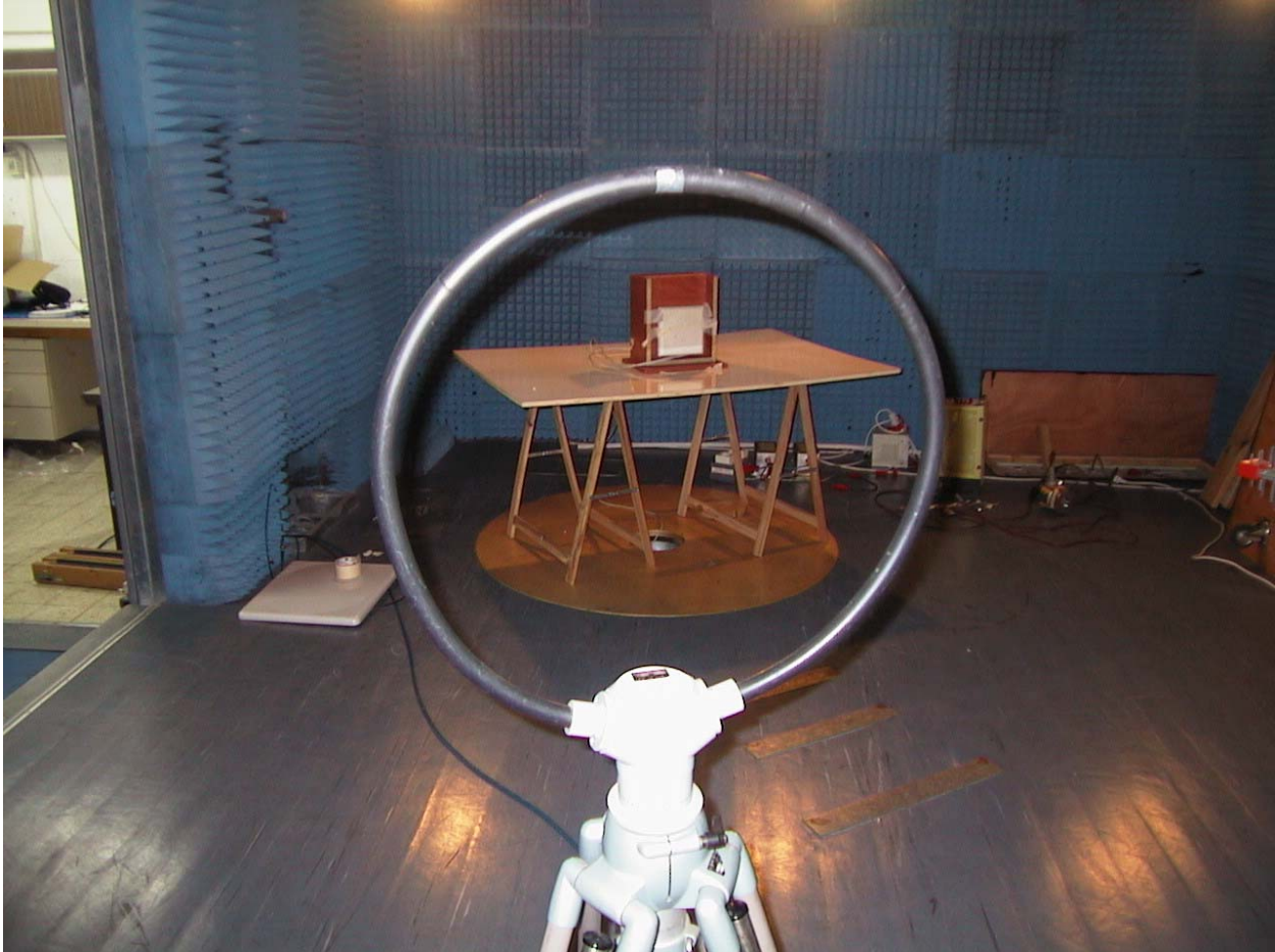
Radiated emission up to 30MHz Setup
