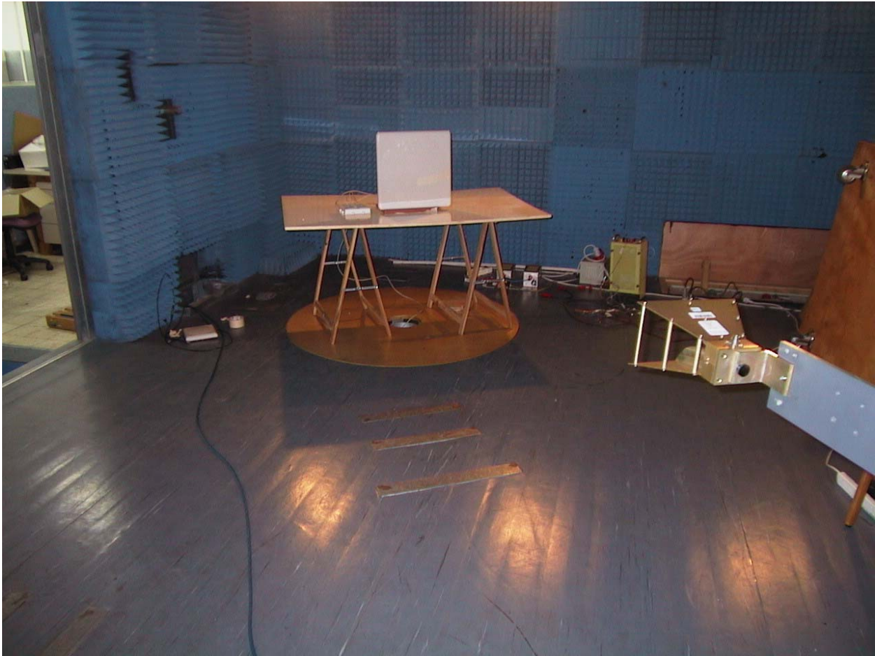
Radiated emission 1GHz – 18GHz Setup
