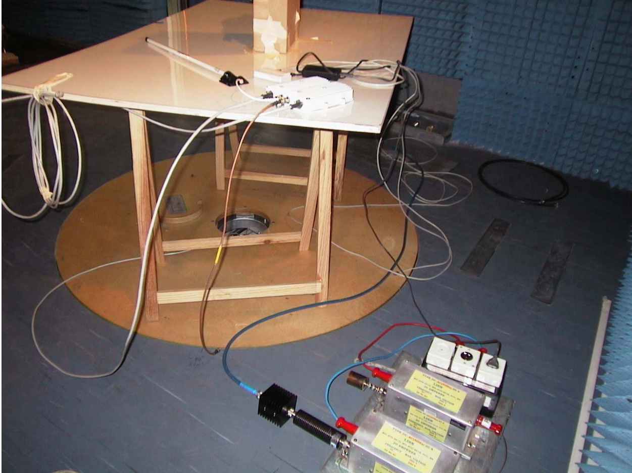
AC Line conducted test set-up picture
