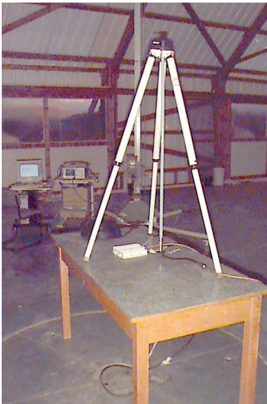
Photograph No.10 Radiated emissions measurement setup view with 12 dBi antenna
