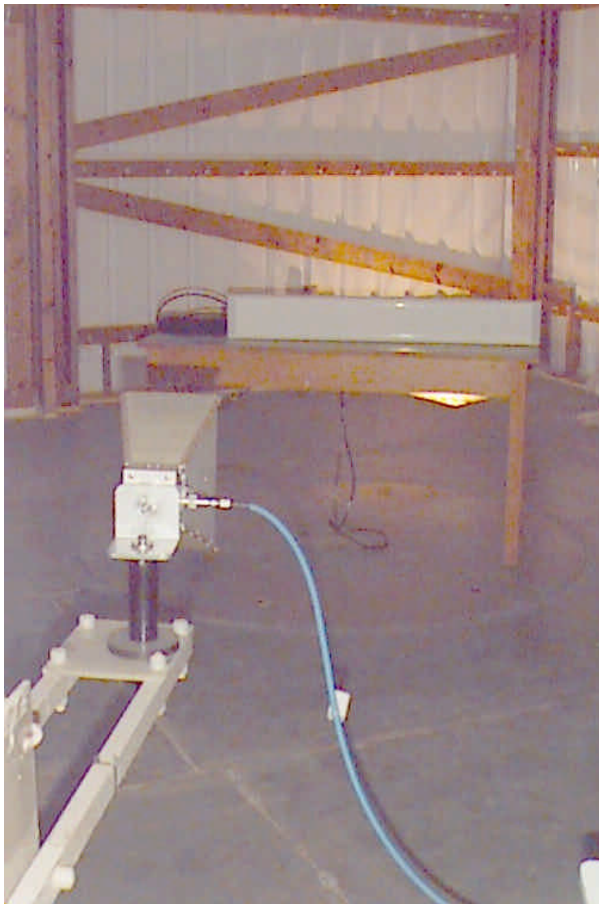
Photograph No.7 Radiated emissions measurement setup view with 17 dBi antenna
