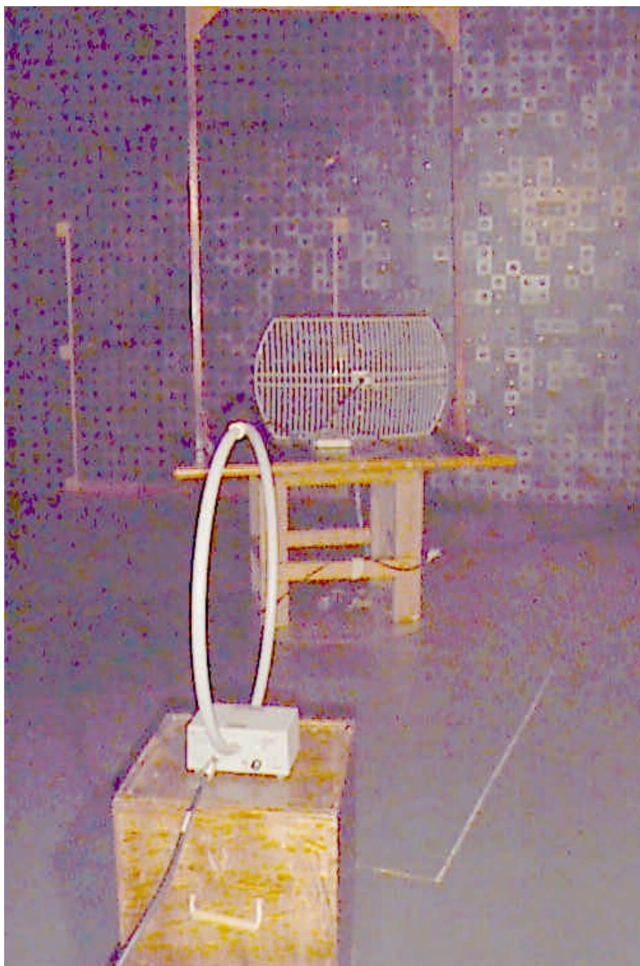
Photograph No.12 Radiated emissions measurement setup view with 24 dBi antenna
