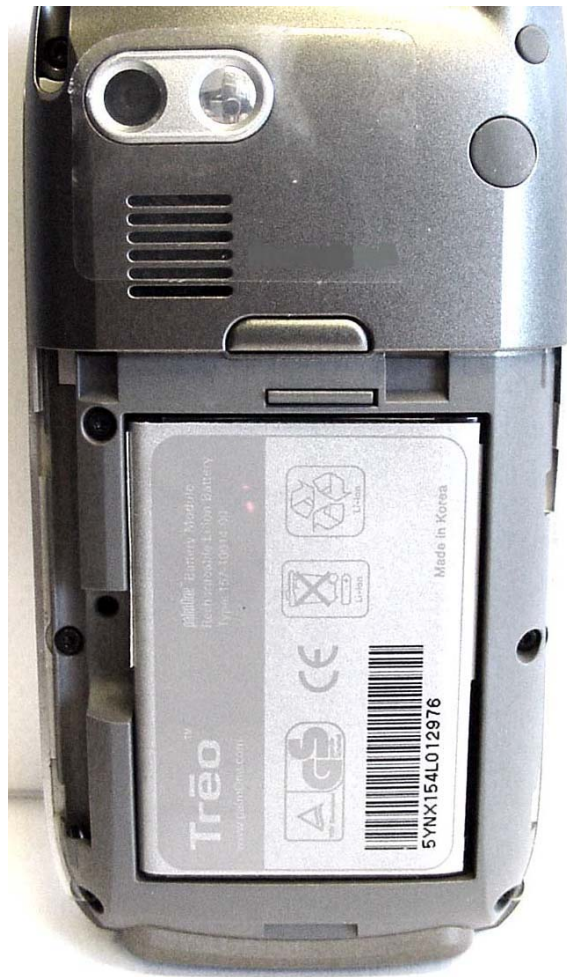
DUT with Lithium-ion Battery
