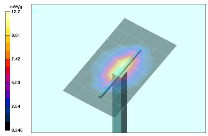
1 g average of 10 measurements: 10.67 mW/g 10 g average of 10 measurements: 5.71 mW/g
