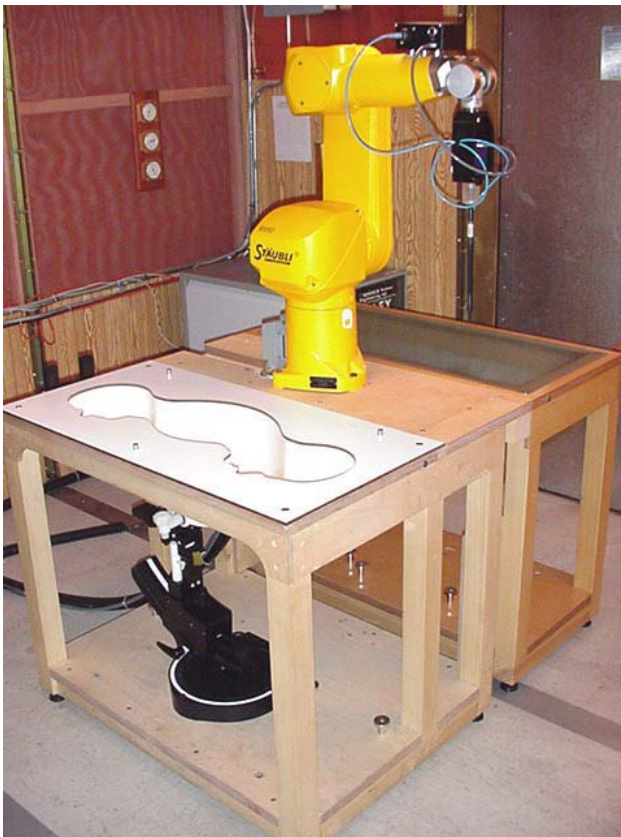
DASY4 Measurement System with SAM Phantom
