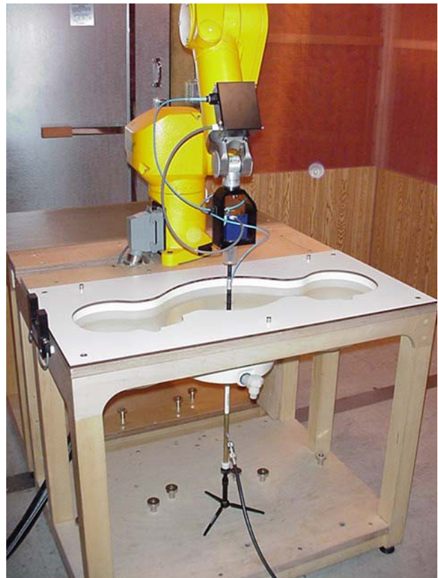
DASY4 Measurement System with SAM Phantom
