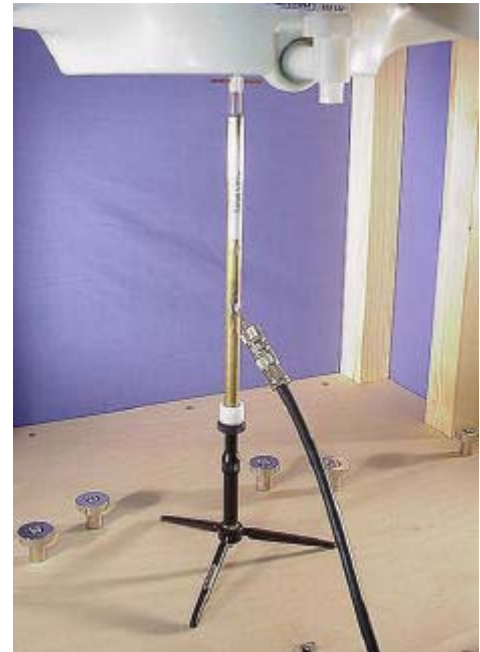
2450MHz System Check Setup Photograph
