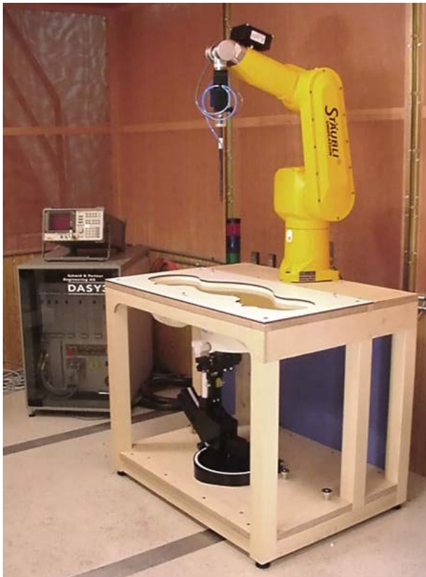
DASY3 SAR Measurement System with SAM phantom
