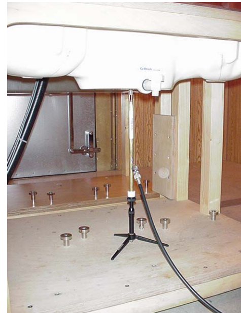
2450MHz Dipole Setup
