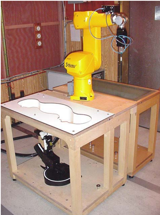
DASY4 Measurement System with SAM Phantom
