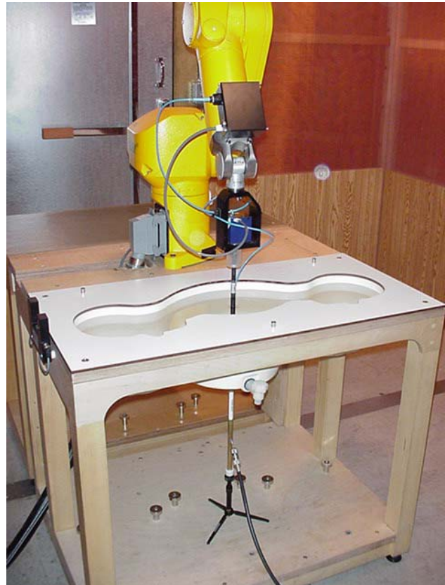
DASY4 Measurement System with SAM Phantom
