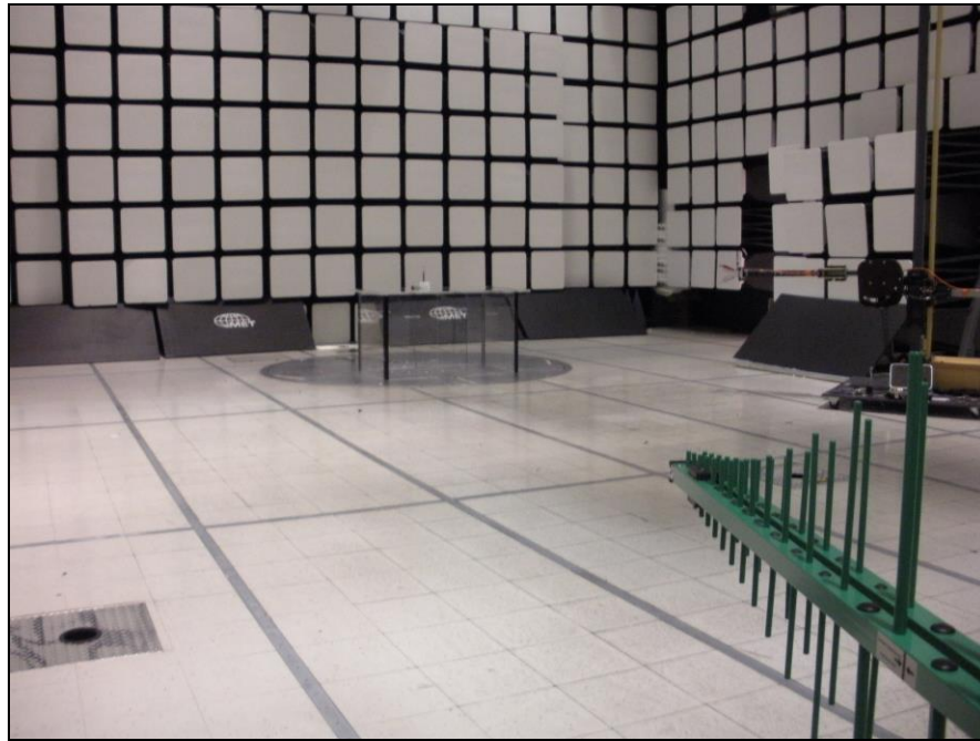
Photograph 2. Radiated Spurious Emissions, Test Setup, 30 MHz – 1 GHz
