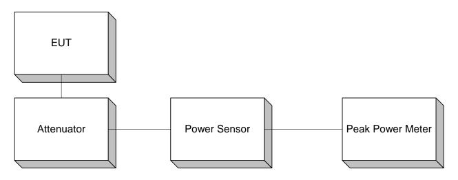
Note: A spectrum analyzer may be substituted for Peak Power Meter given that the measurement bandwidth is sufficient to capture the 60 dB bandwidth of the transmitter.
