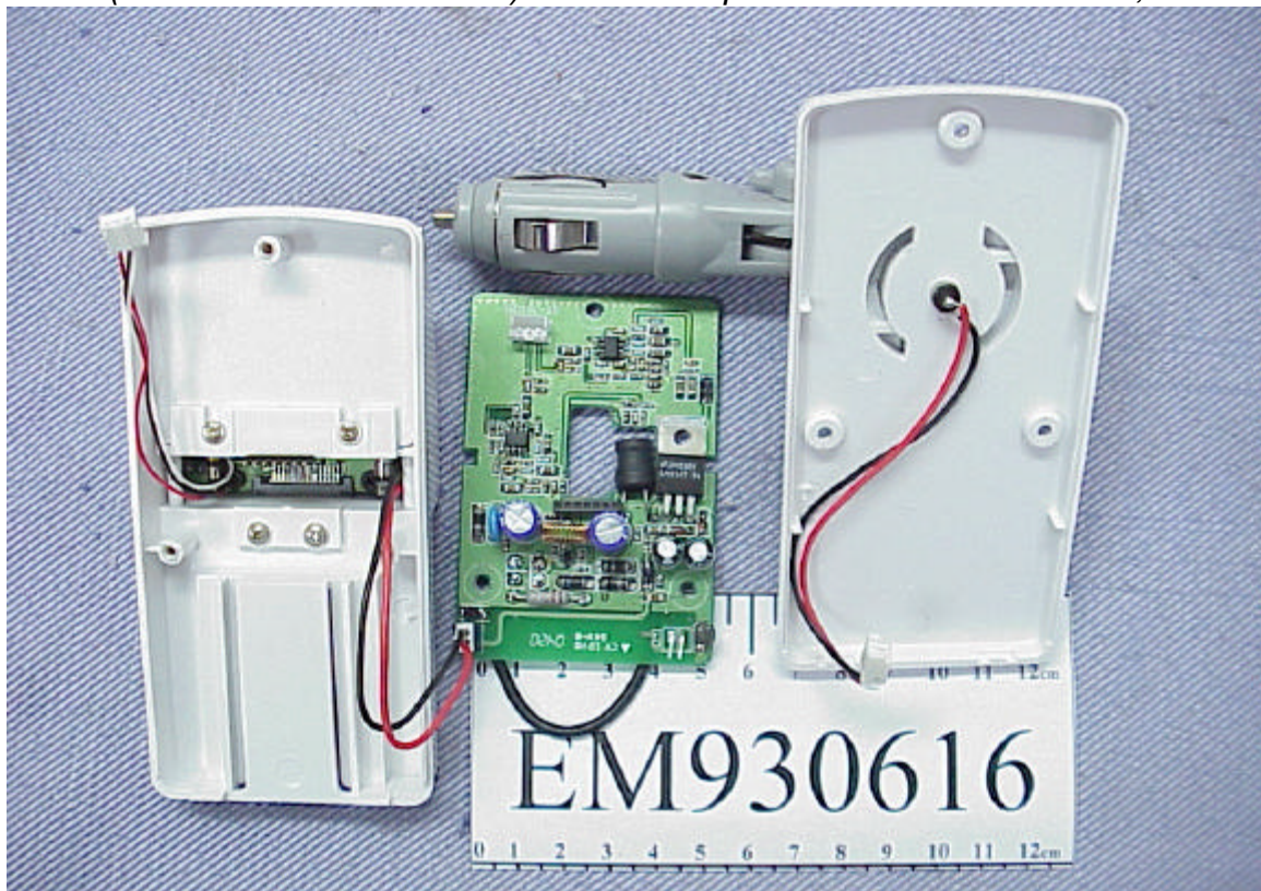
Photo 6 (Holder/ Transmitter Base) Remove Top Cover and Bottom Cover, Internal View
