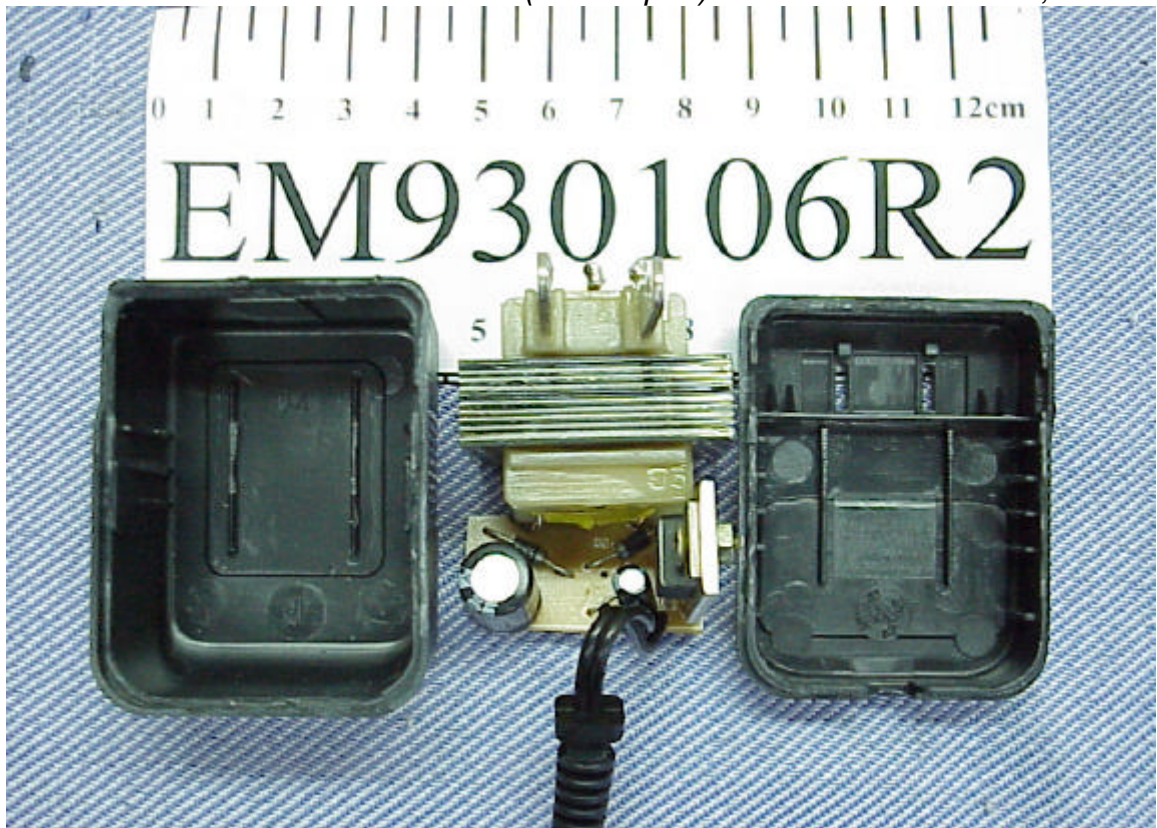
Photo 16 (AC Adapter) Remove Case Covers, Internal View
