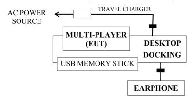
3.2.1.3. EUT with Desktop and Link to PC, Power with USB Port from PC
