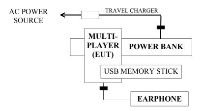
3.2.1.5. EUT with Power Bank, Power with Saver Charger from DC Power
