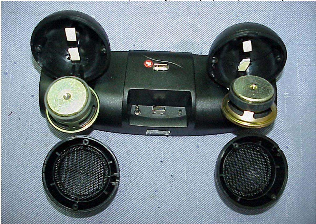
Photos 54 (Accessory, Desktop Speaker) Internal Speakers View
