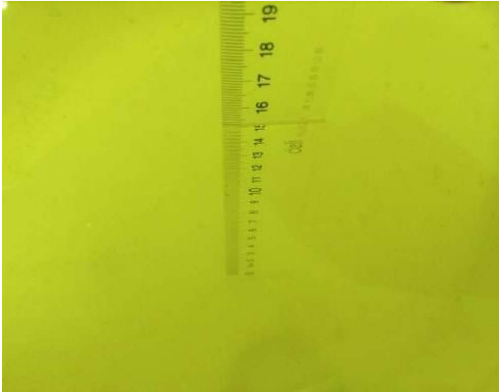
Picture 7-5: Liquid depth in the Flat Phantom (2450 MHz Head)
