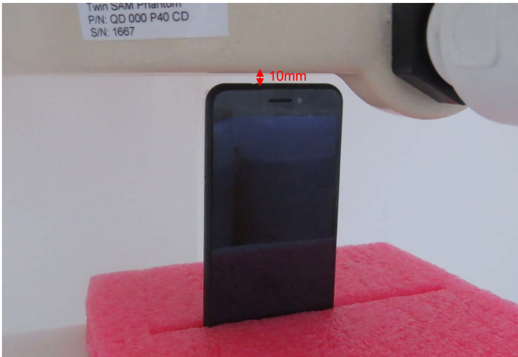
Picture 14: Top Side, the distance from handset to the bottom of the Phantom is 10mm
