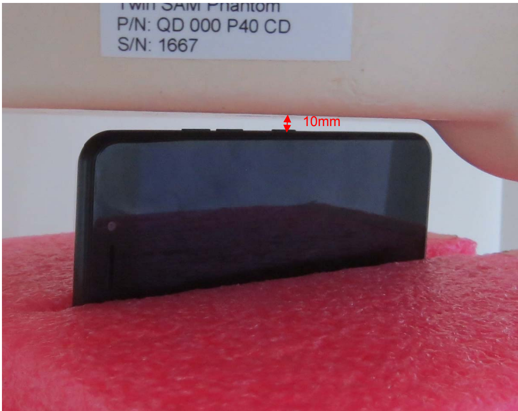
Picture 13: Right Side, the distance from handset to the bottom of the Phantom is 10mm
