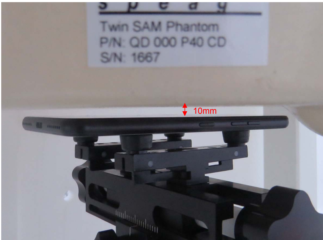
Picture 12: Front Side, the distance from handset to the bottom of the Phantom is 10mm
