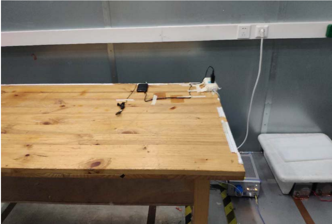
Picture 2 Conducted Emission Test Setup
