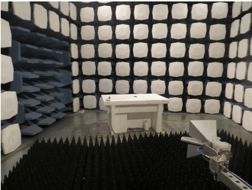
Picture 1: Radiated Spurious Emissions Test setup
