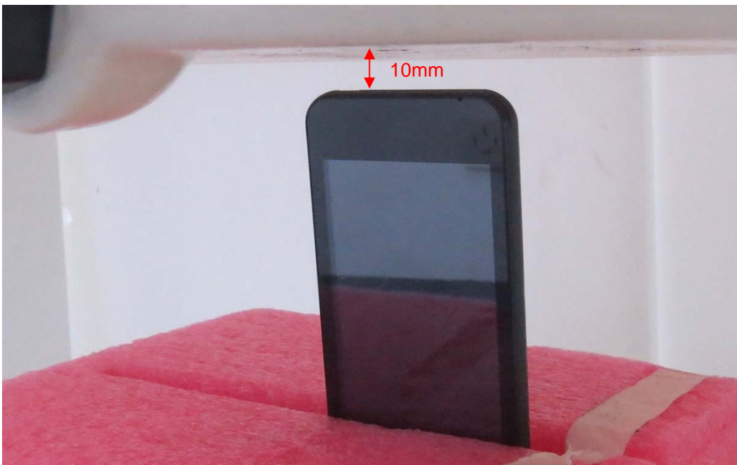
Picture 10: Bottom Side, the distance from handset to the bottom of the Phantom is 10mm
