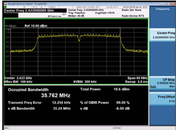
802.11n(HT40), Carrier frequency (MHz): 2437
