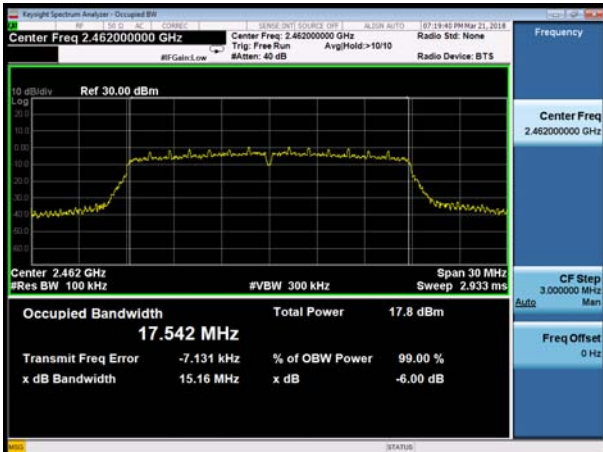
802.11n(HT20), Carrier frequency (MHz): 2462
