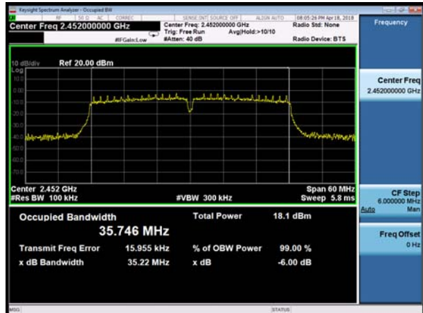
802.11n(HT40), Carrier frequency (MHz): 2452
