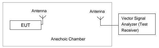
The measurement is made according to KDB 789033
