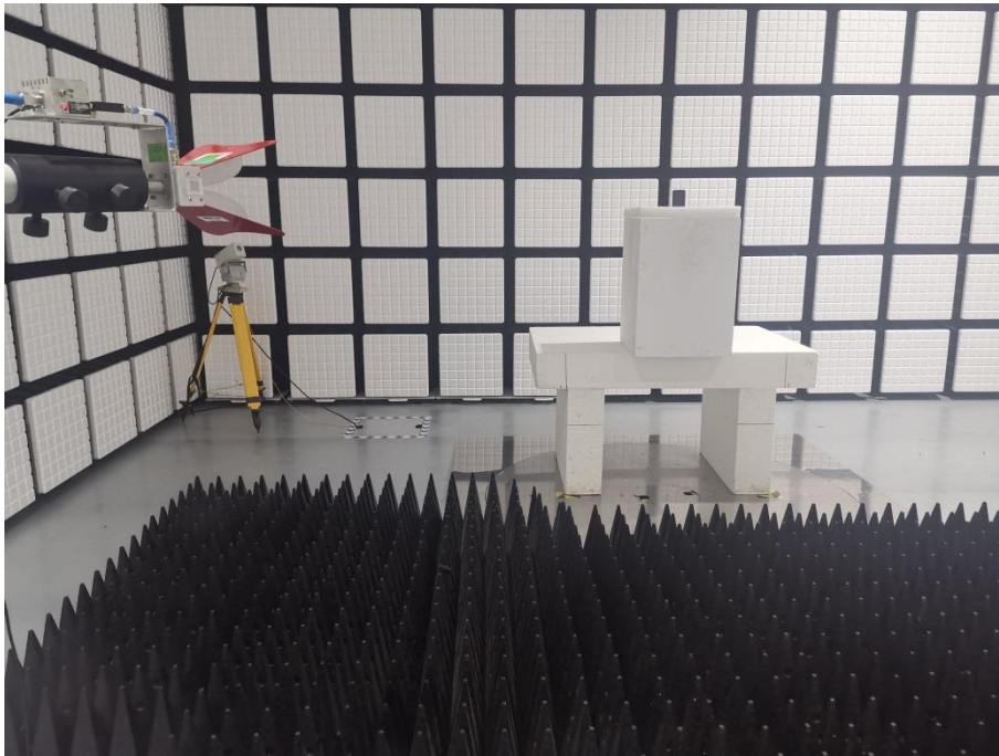
Description: Radiated Emission Test Setup (1 GHz -18GHz)
