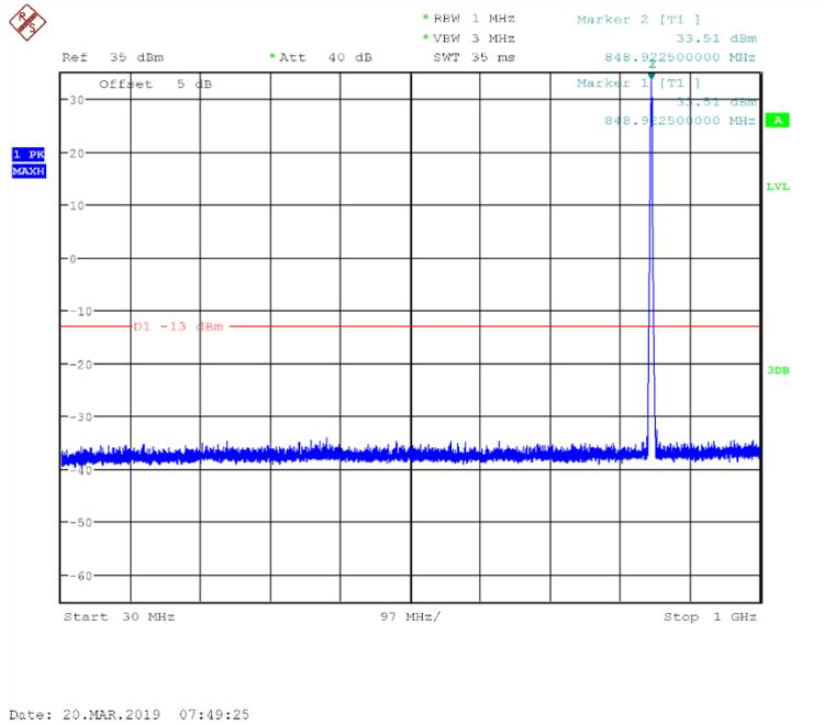
Fig.69 Channel 251: 30MHz~1GHz
