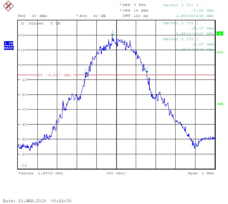
Fig.35 Channel 512- Emission Bandwidth (-26dBc BW)
