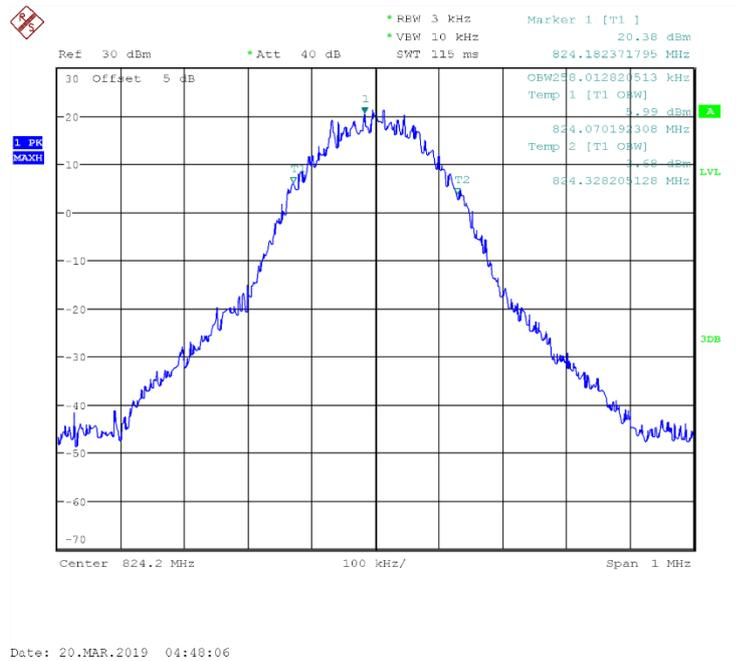
Fig.8 Channel 128-Occupied Bandwidth (99%)
