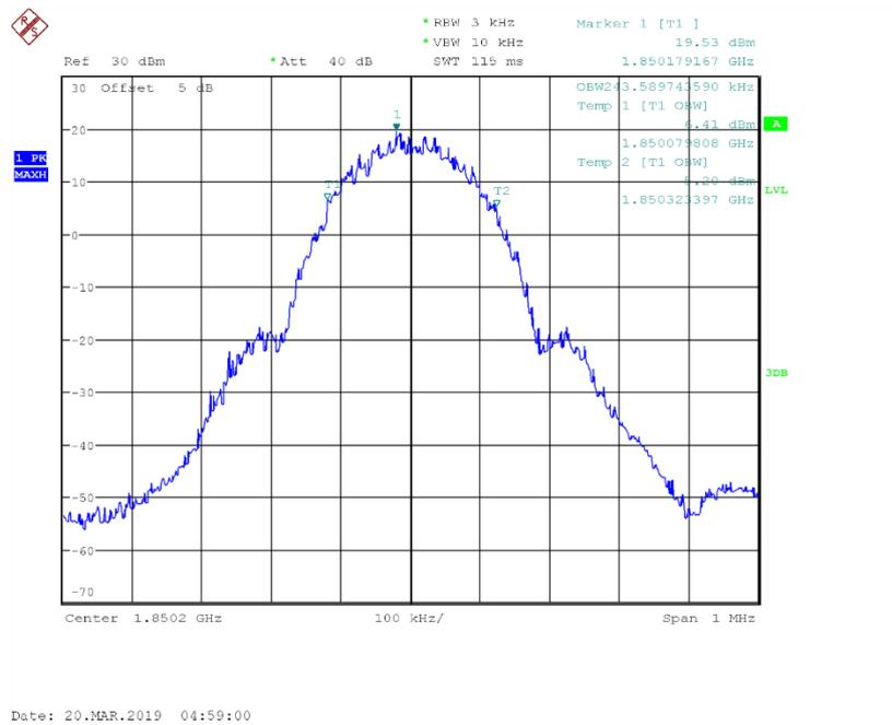
Fig.14 Channel 512-Occupied Bandwidth (99%)
