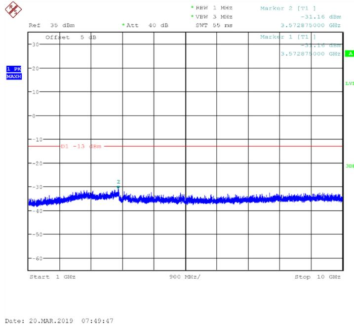
Fig.70 Channel 251: 1GHz~10GHz
