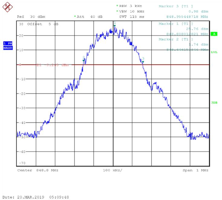
Fig.27 Channel 251- Emission Bandwidth (-26dBc BW)
