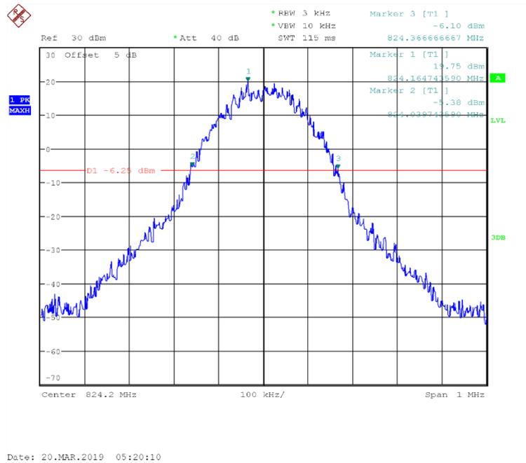
Fig.32 Channel 128- Emission Bandwidth (-26dBc BW)
