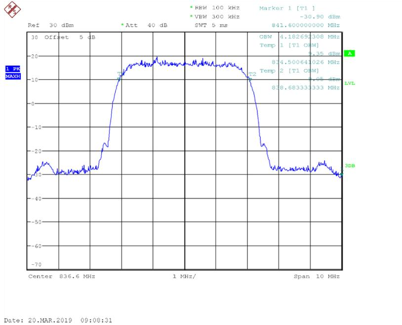
**Fig.22 Channel 4183-Occupied Bandwidth (99%)**
