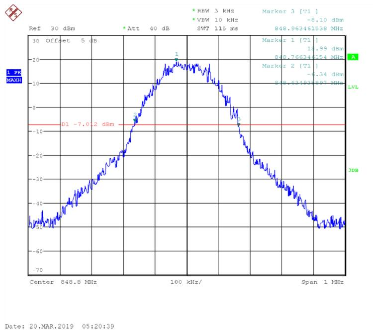
Fig.33 Channel 251- Emission Bandwidth (-26dBc BW)
