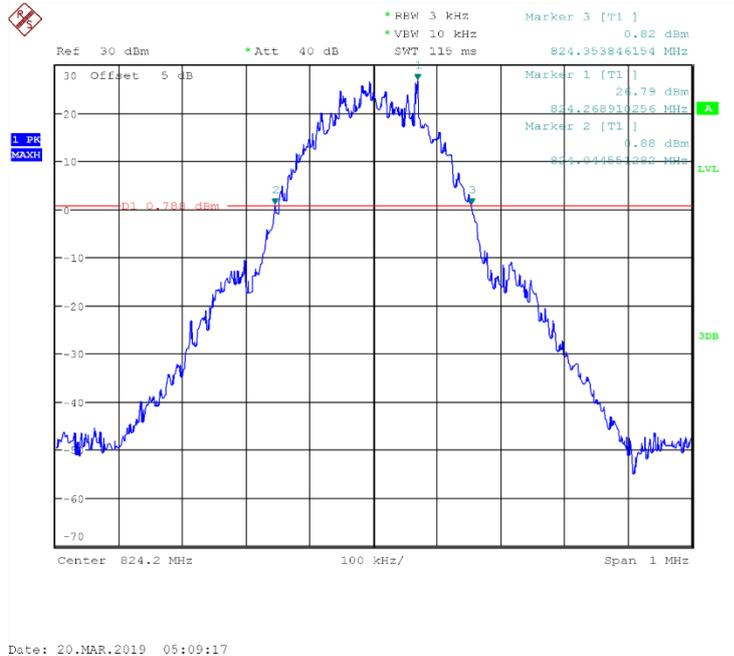
Fig.26 Channel 128- Emission Bandwidth (-26dBc BW)
