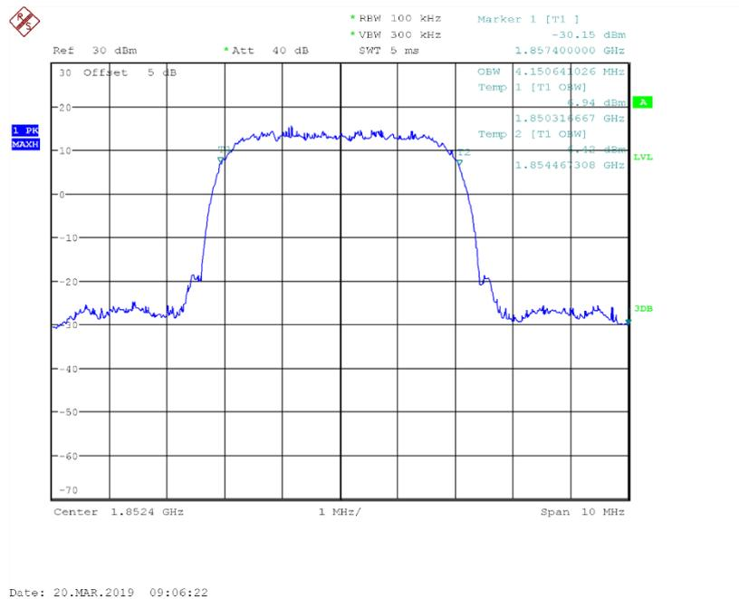
Fig.20 Channel 9262-Occupied Bandwidth (99%)
