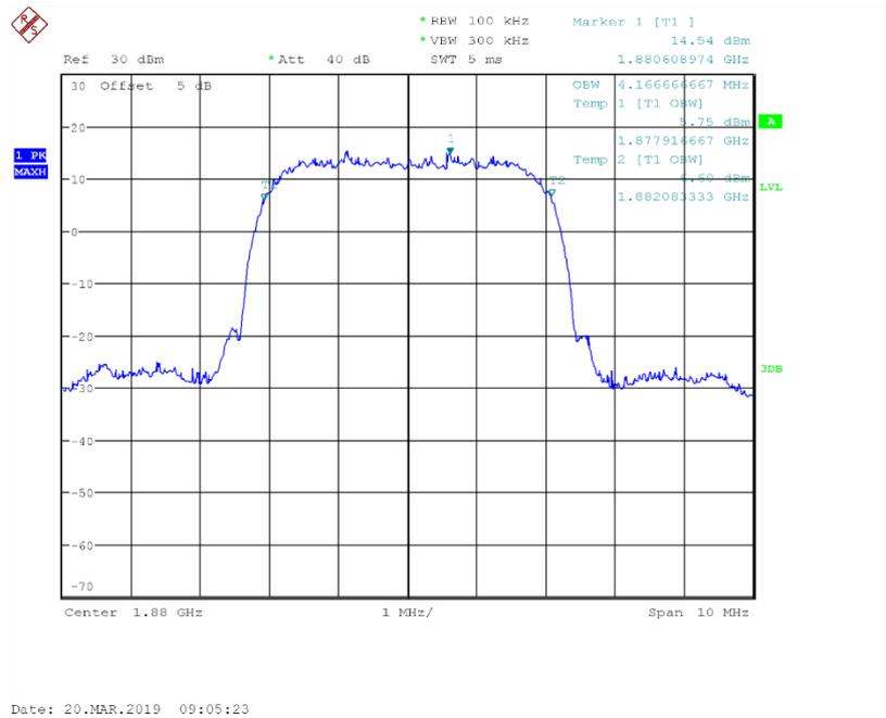
Fig.19 Channel 9400-Occupied Bandwidth (99%)
