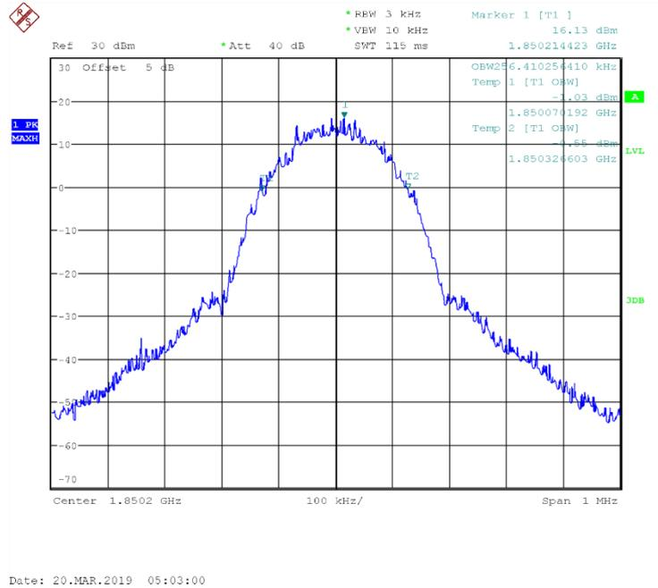
Fig.17 Channel 512-Occupied Bandwidth (99%)
