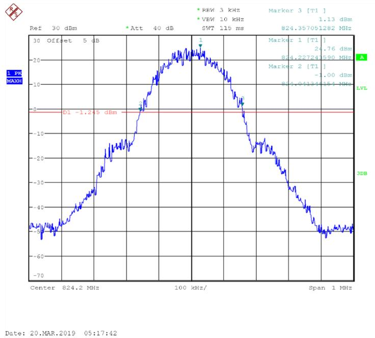
Fig.29 Channel 128- Emission Bandwidth (-26dBc BW)
