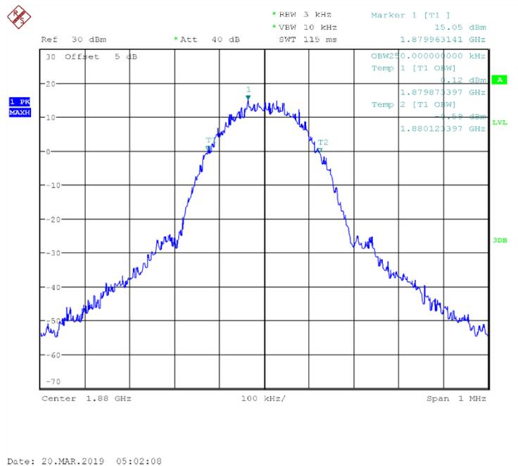
Fig.16 Channel 661-Occupied Bandwidth (99%)
