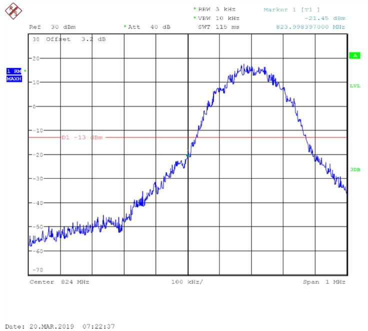
Fig.53 Channel 128- LOW BAND EDGE BLOCK
