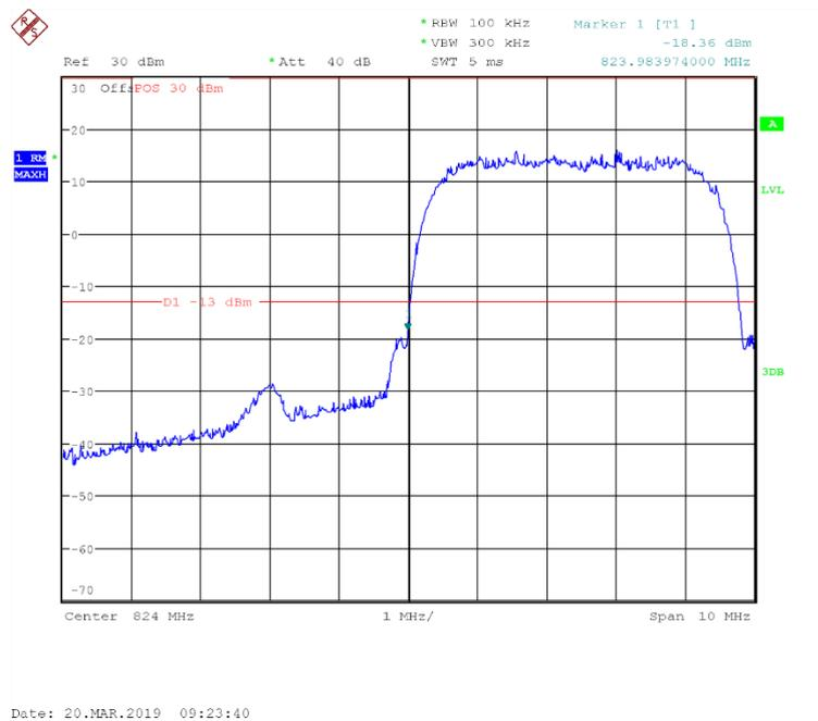
Fig.63 Channel 4132- LOW BAND EDGE BLOCK
