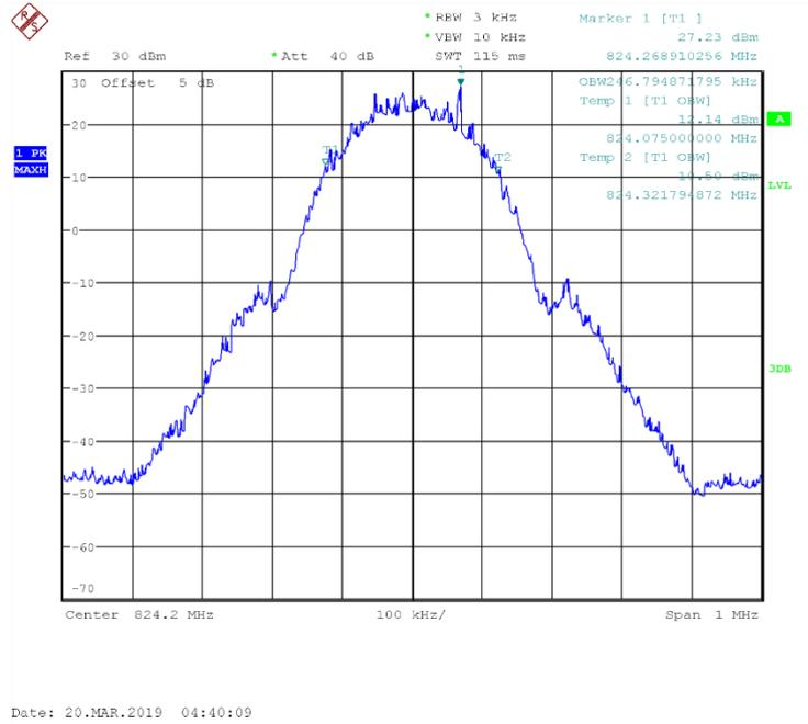
Fig.2 Channel 128-Occupied Bandwidth (99%)
