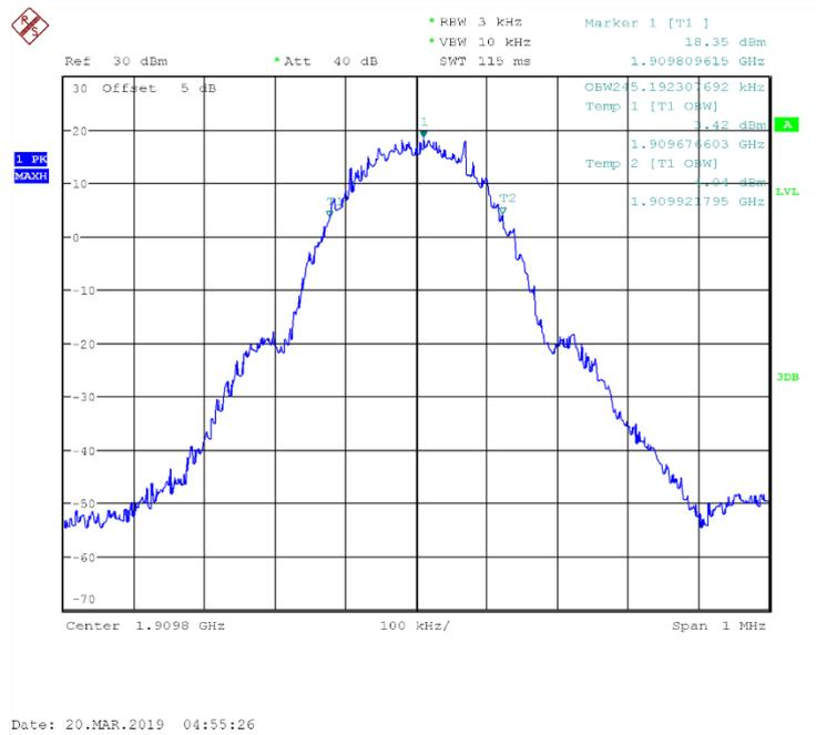
Fig.12 Channel 810-Occupied Bandwidth (99%)
