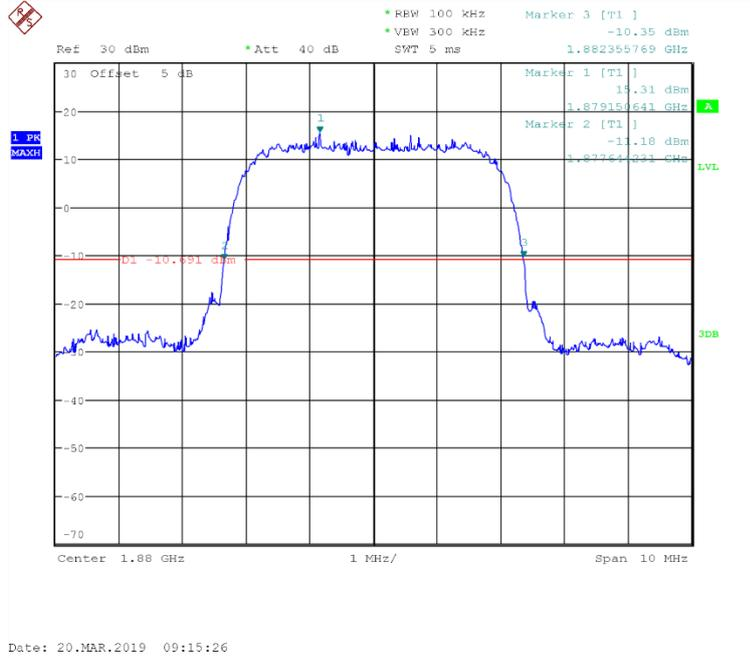
Fig.43 Channel 9400- Emission Bandwidth (-26dBc BW)
