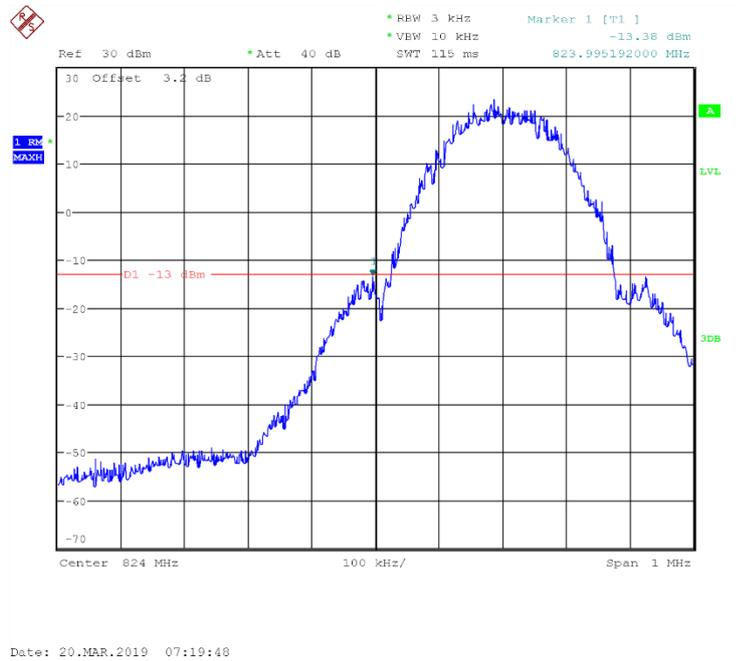
Fig.51 Channel 128- LOW BAND EDGE BLOCK
