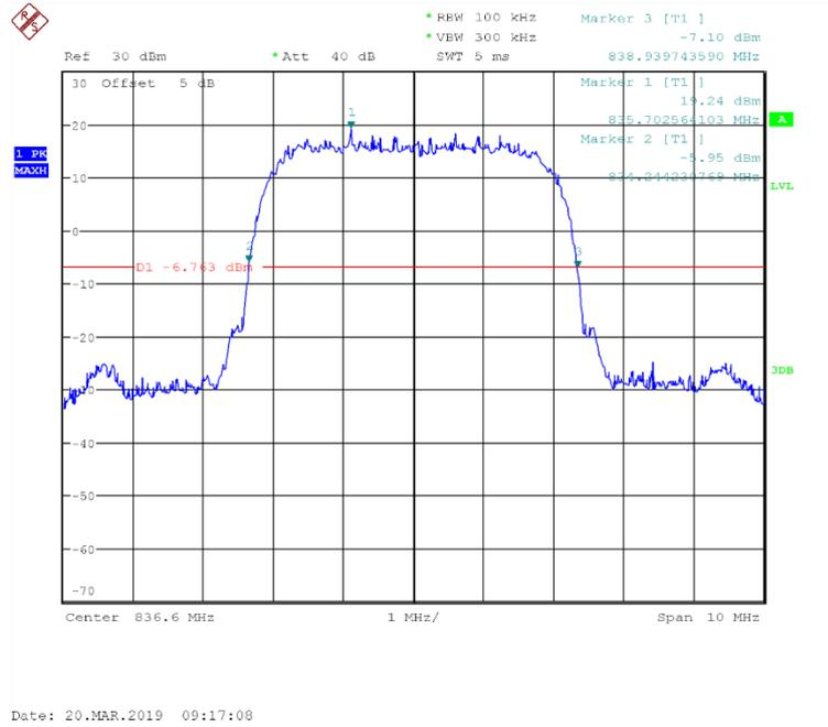
Fig.46 Channel 4183- Emission Bandwidth (-26dBc BW)
