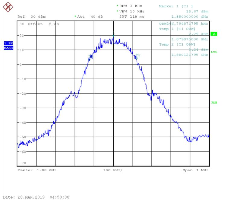
Fig.13 Channel 661-Occupied Bandwidth (99%)
