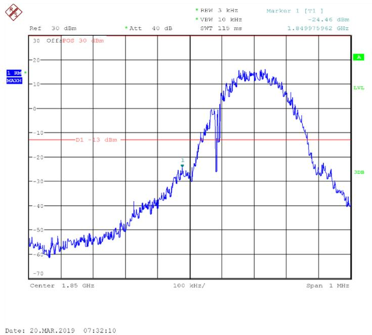
Fig.59 Channel 512- LOW BAND EDGE BLOCK
