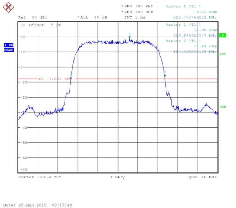
Fig.47 Channel 4132- Emission Bandwidth (-26dBc BW)
