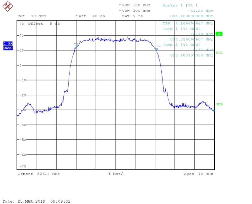
**Fig.23 Channel 4132-Occupied Bandwidth (99%)**
