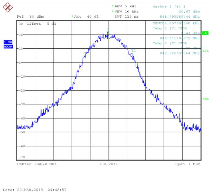
Fig.9 Channel 251-Occupied Bandwidth (99%)
