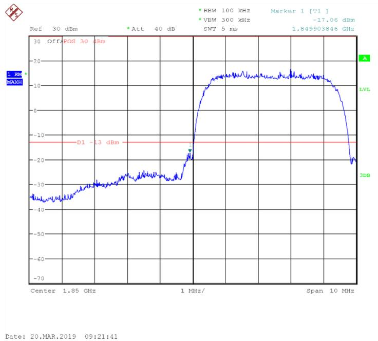
Fig.61 Channel 9262- LOW BAND EDGE BLOCK
