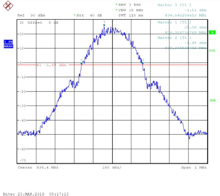
Fig.28 Channel 189- Emission Bandwidth (-26dBc BW)
