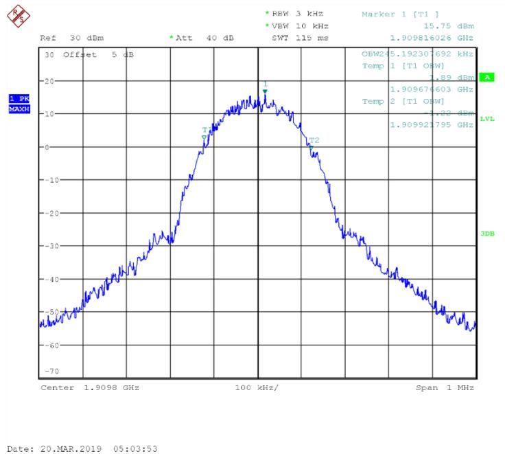
Fig.18 Channel 810-Occupied Bandwidth (99%)
