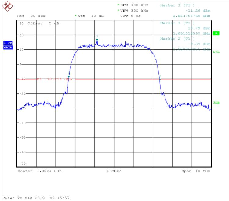
Fig.44 Channel 9262- Emission Bandwidth (-26dBc BW)
