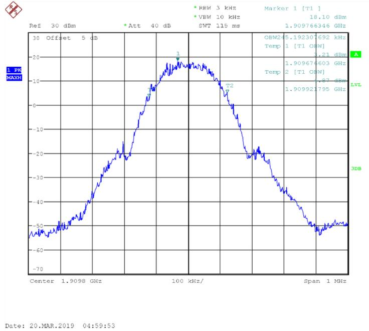
Fig.15 Channel 810-Occupied Bandwidth (99%)
