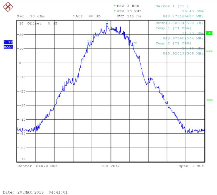
Fig.3 Channel 251-Occupied Bandwidth (99%)
