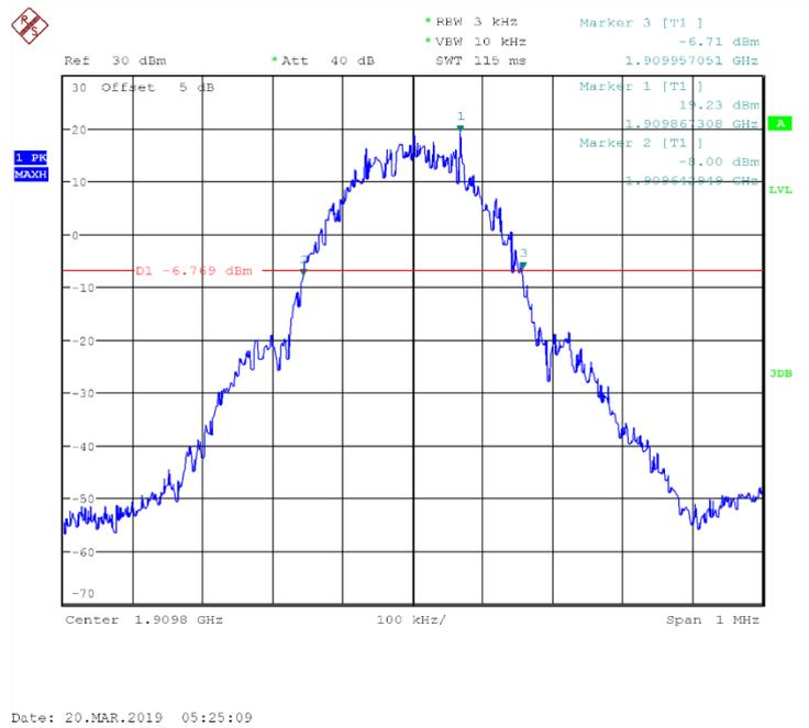
Fig.36 Channel 810- Emission Bandwidth (-26dBc BW)
