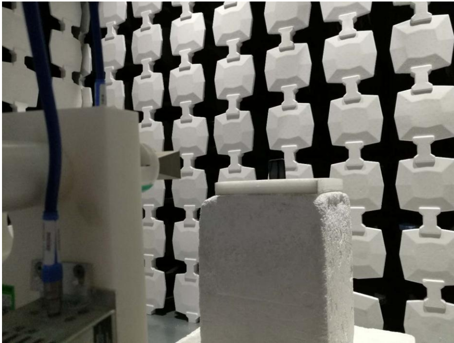
Description: Radiated Emission Test Setup (Above 18GHz)
