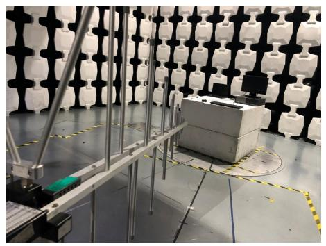
Description: Radiated Emission Test Setup
