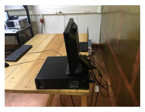
Test Mode: Mode 1 Description: Front view of Radiated Emission Test Setup
