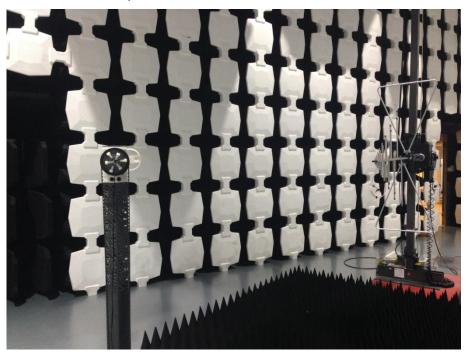
Description: Substitution Antenna for ERP Test
