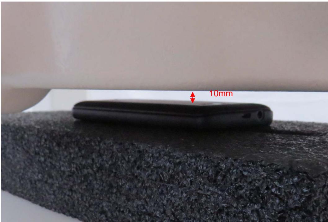
Picture 2: Back Side, the distance from handset to the bottom of the Phantom is 10mm
