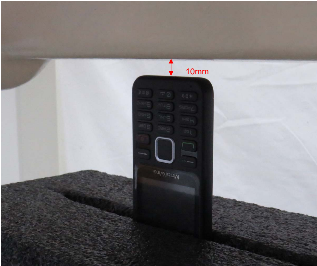
Picture 3: Bottom Edge, the distance from handset to the bottom of the Phantom is 10mm
