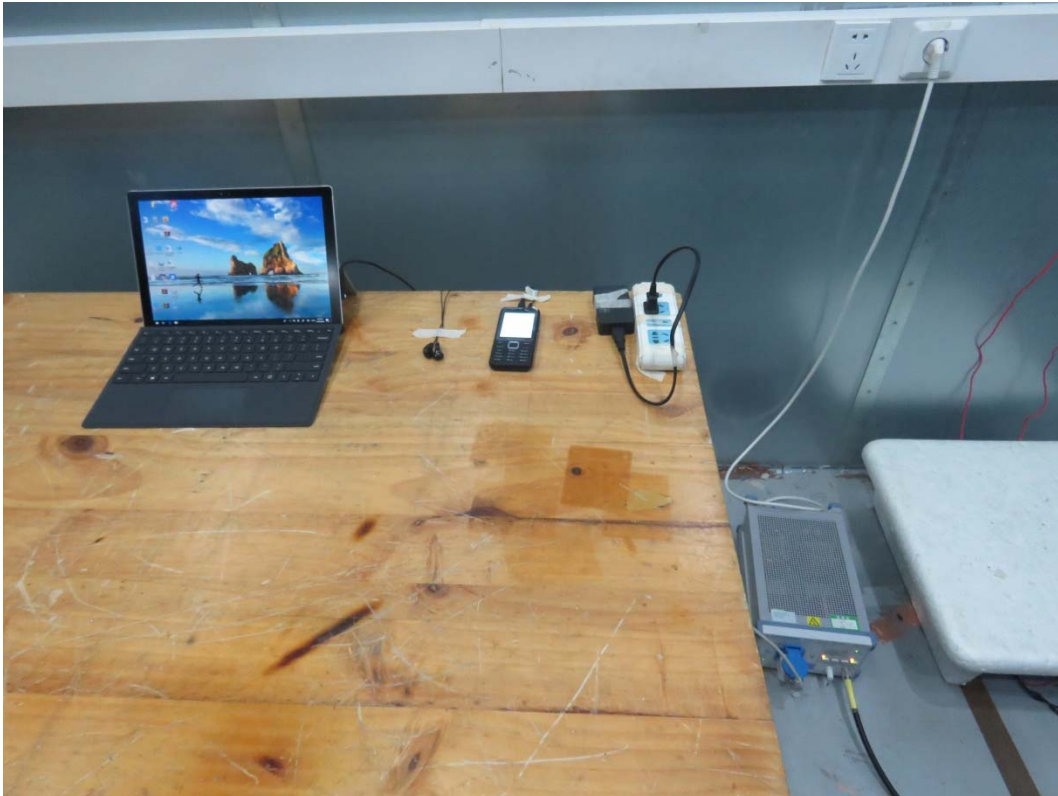
Picture 2 Conducted Emission Test Setup
