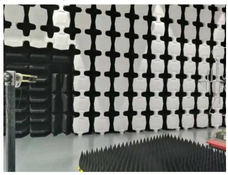
Description: Substitution Antenna for ERP Test
