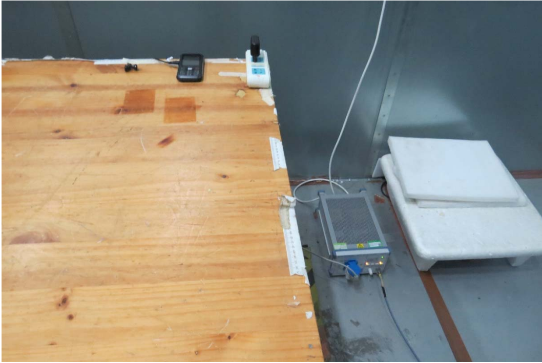
Picture 3 Conducted Emission Test Setup
