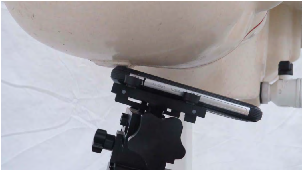
Picture 9: Right Hand Tilt 15 Degree Position
