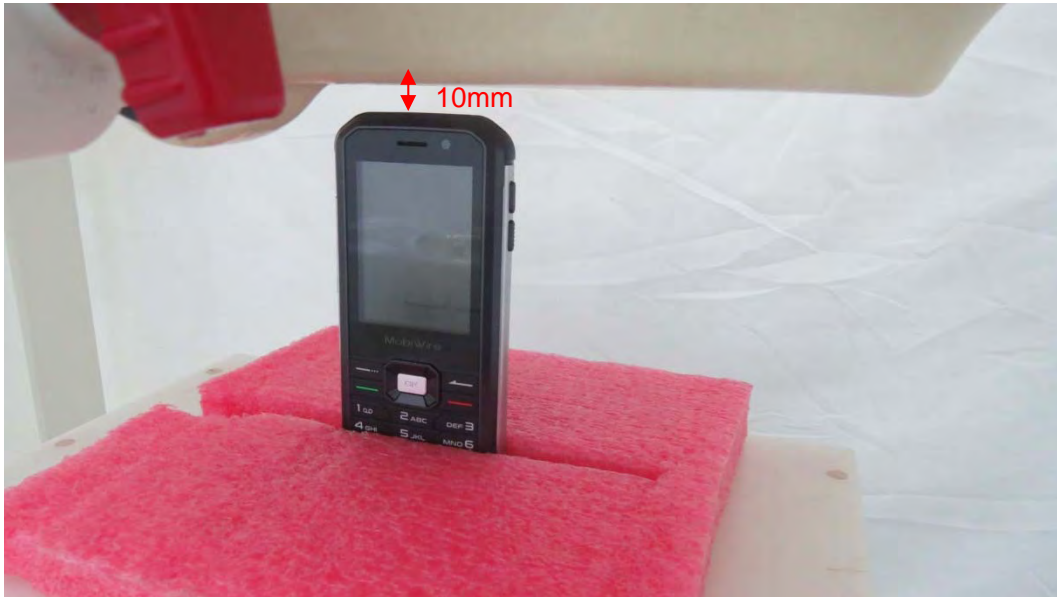
Picture 16: Top Side, the distance from handset to the bottom of the Phantom is 10mm
