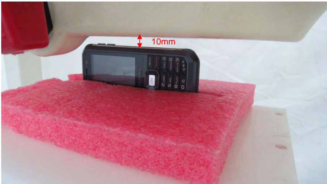
Picture 15: Right Side, the distance from handset to the bottom of the Phantom is 10mm
