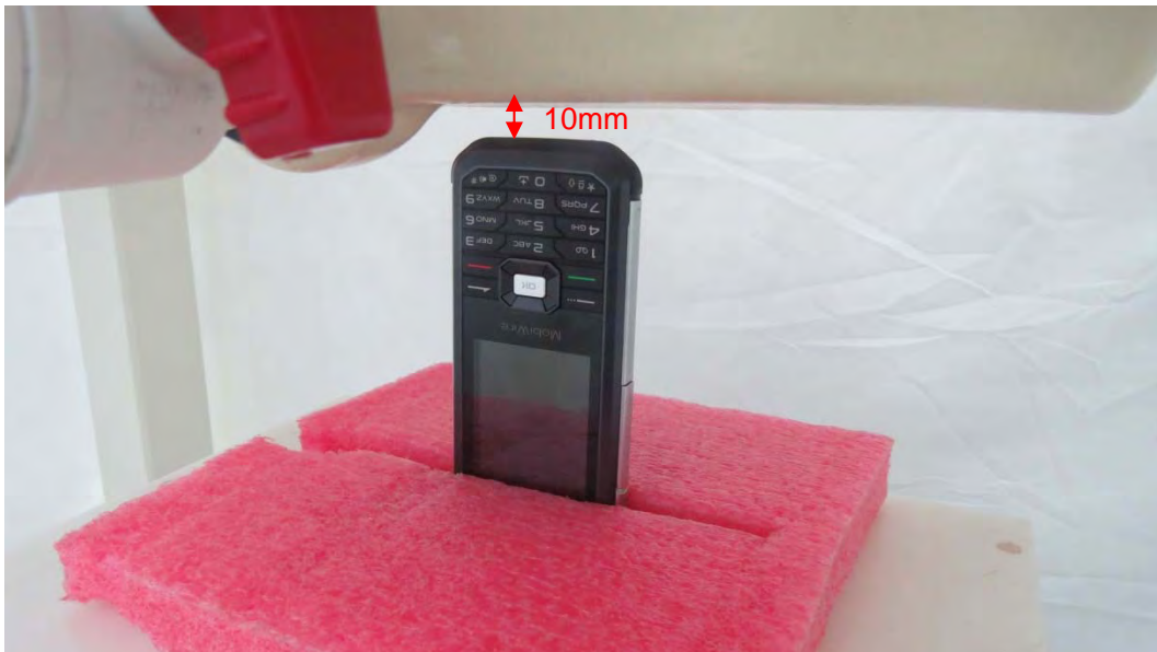
Picture 17: Bottom Side, the distance from handset to the bottom of the Phantom is 10mm
