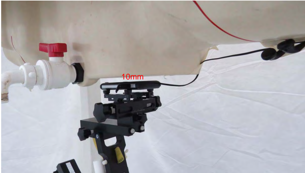
Picture 18: Back Side, the distance from handset to the bottom of the Phantom is 10mm
