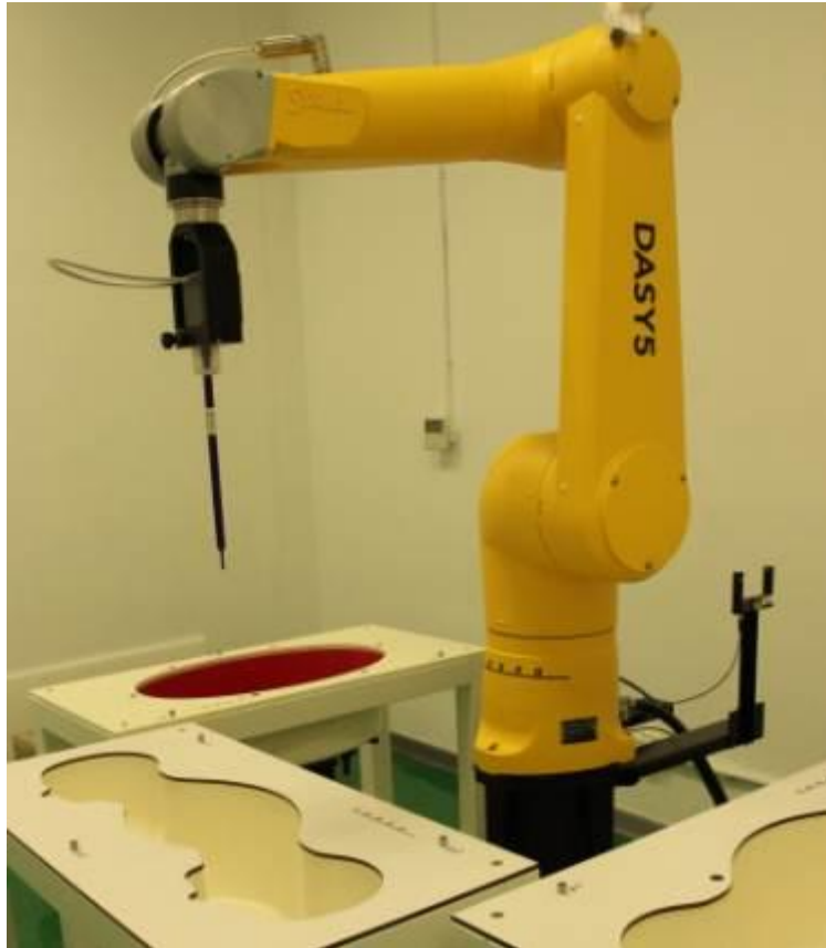
Picture 8-7: Specific Absorption Rate Test Layout
