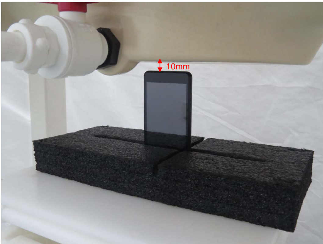
Picture 12: Bottom Edge, the distance from handset to the bottom of the Phantom is 10mm
