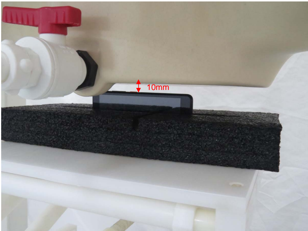
Picture 10: Right Side, the distance from handset to the bottom of the Phantom is 10mm
